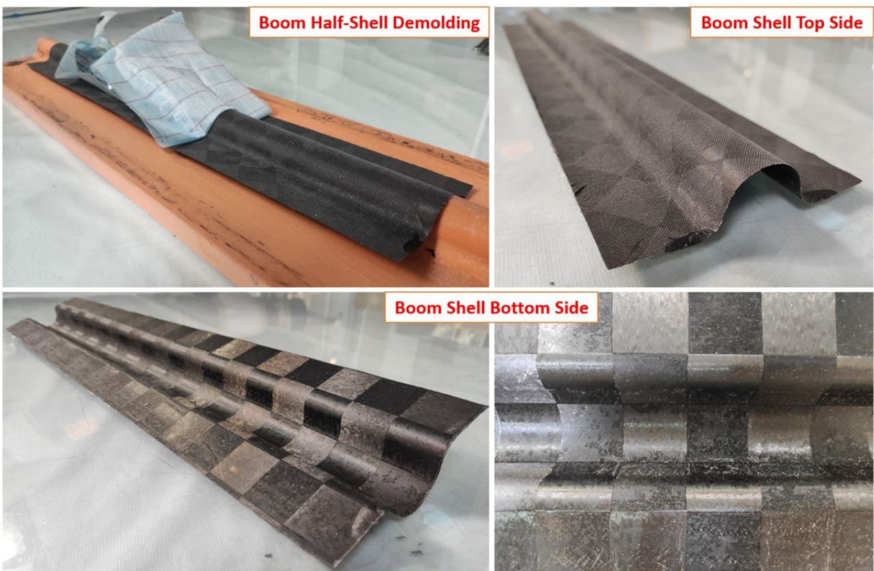
Figure 5.22: Demolding of a boom half-shell and closeup pictures[142].
