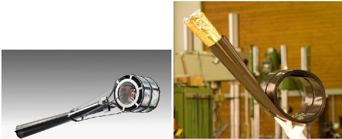
Figure 5.3: Electrically driven boom tip (left) and inflatable boom (right) from [128]. Reproduced with permission.
