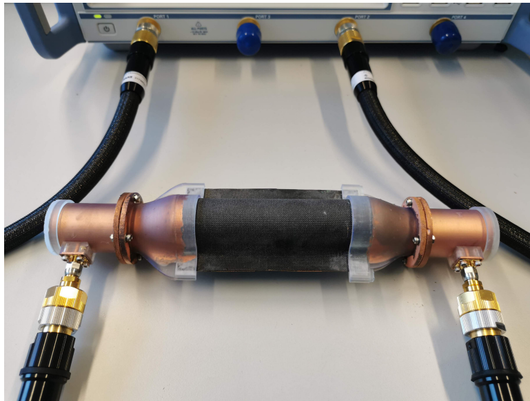
Figure 5.32: Measurement Setup of the CTM waveguide prototype with TE mode coaxial adapters.
