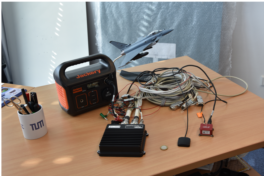
Figure 4.1: The DuraCOR 311 with the Ellipse sensor and a GPS antenna plugged in.
