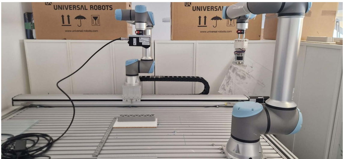
Figure 3.15: General scanning and printing position
