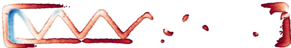
Figure 6.17: Final layer height deviation map dry
