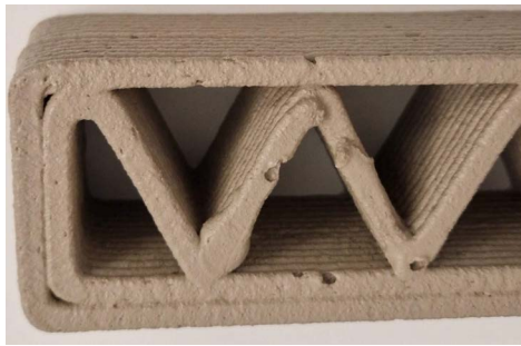
Figure 6.6: Intermediate layer with air bubble
