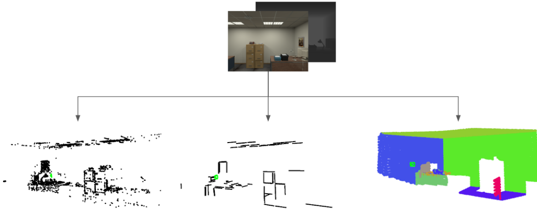
Figure 2.1 Feature reconstructed from a pair of RGB-D images. In the bottom row, from left to right, there are point, line and plane primitives.
