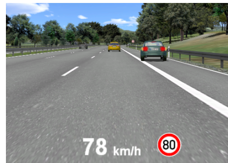
Fig. 1. Investigated perspective in this study. A stranded vehicle causes an MRM of the AV that drives in front of the ego vehicle. The picture was extracted from the simulation software SILAB.
