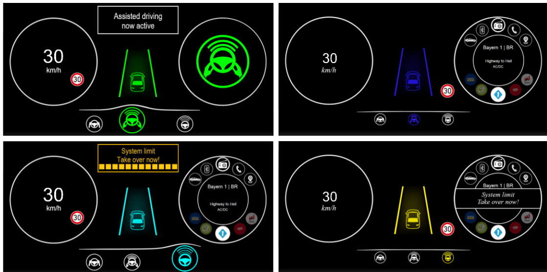
Figure 5.5 Excerpts of the HMI concepts ( left: HC-HMI; right: LC-HMI ) in the IC. Top : L2 has just been activated. Bottom : Second stage of the warning cascade during the RtI_{20s} . Note . The second stage of the warning cascade during the RtI_{20s} in the HC-HMI indicates a countdown (one box disappears per second). The warning is supplemented with yellow LED lights flashing on the steering wheel and a warning sound with low criticality.
