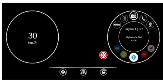
Feedback for handling error ( MOD button has no function in L0)
