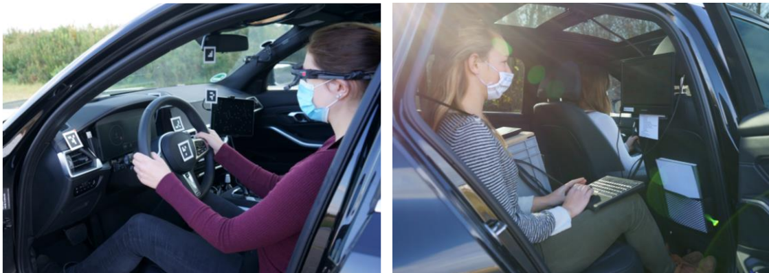
Figure 5.7 Photos of the experimental setup. Left: The participant wears the eye-tracking system Dikablis Glasses 3 by Ergoneers. Right: The experimenter gives instructions, triggers events, and controls the data recording.
