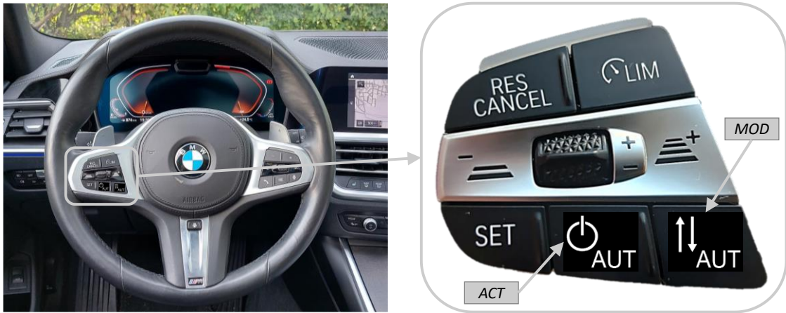
Figure 5.2 Left: Position of the control buttons on the steering wheel. Right: Control buttons ACT and MOD and their respective icons.
