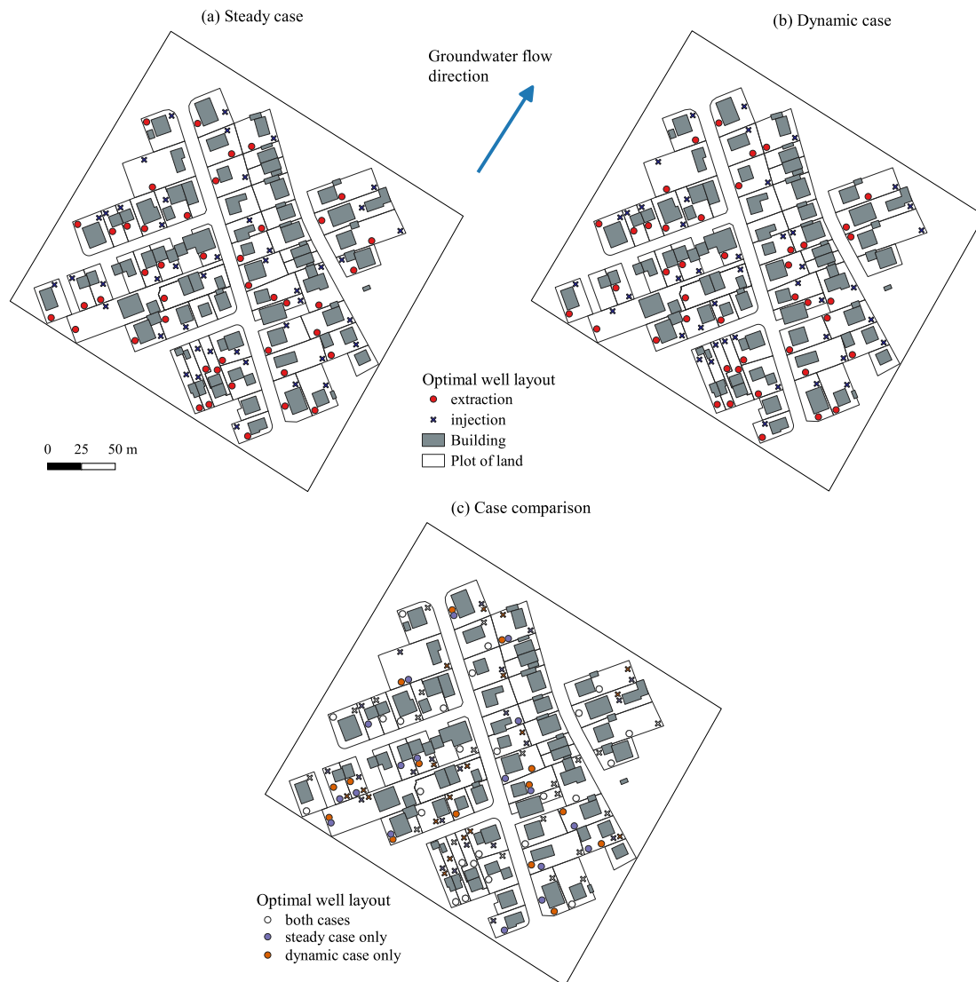
Fig. 6. Optimal well locations: (a) The steady case. (b) The dynamic case. (c) Comparison between two cases.
