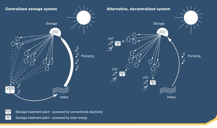
A concept for a decentralized wastewater system developed with the residents of the city of Leh. The water is reused locally, such as to cultivate vegetables or flush toilets. This type of system would reduce demand for fresh water, cut the waste stream, save energy and help to grow food locally.
