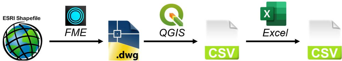
Figure 71: The procedure followed for the data conversion from ESRI Shapefile to CSV.
