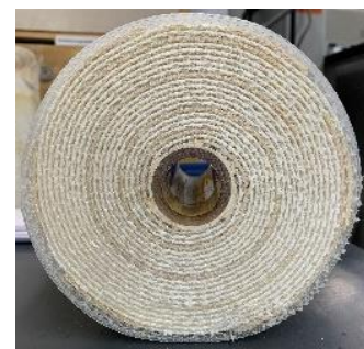
Figure 1-11. Illustration of an industrial-scale SWM (a) (Hartinger et al. 2019b) and its front-view (b).
