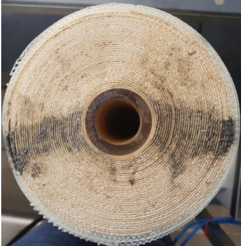
Figure 8-2. The membrane module was modified by adding glue dots (see black areas) radially along the membrane diameter.
