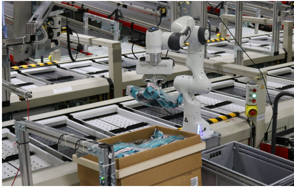
Fig. 1. Franka Emika robot in the logistics facility
