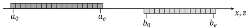
Figure 5-3: The unidimensional projections of two areas if there is no overlap [Sic-2021a]
