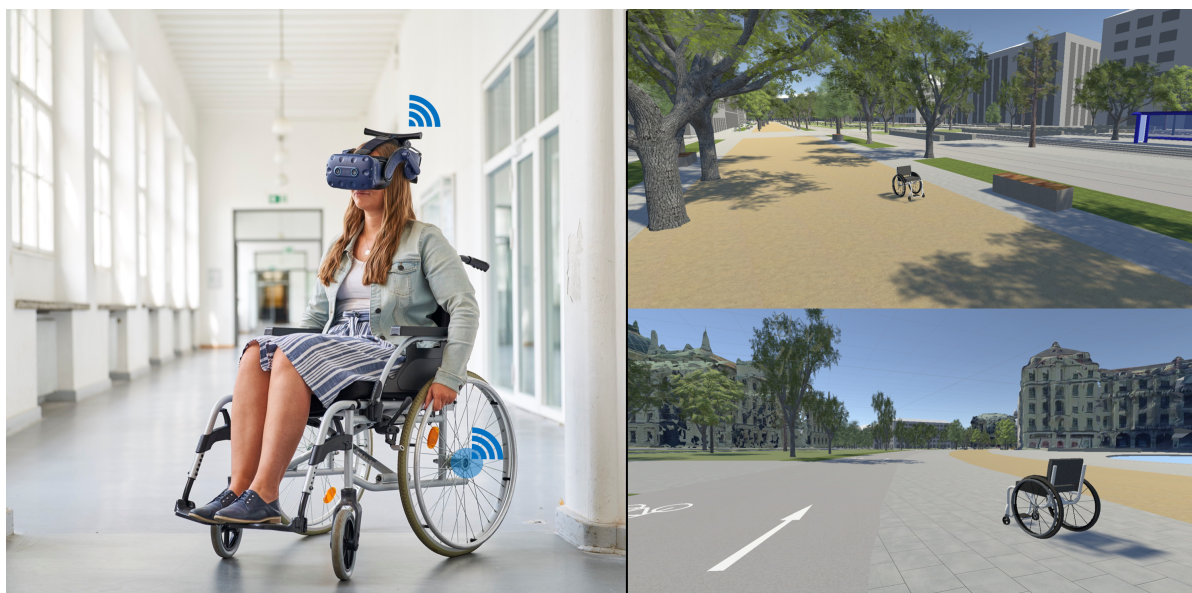
Figure 1: Wheelchair Simulator (left: wheelchair simulator setup, right: virtual model in Unity 3D)
