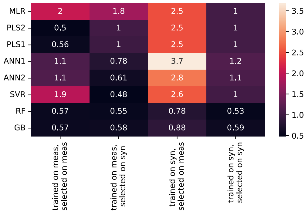
Figure 60: Sum of the scaled-MAE for all models, training datasets, and selection modes evaluated on the additional reduced measurement dataset with five variables.
