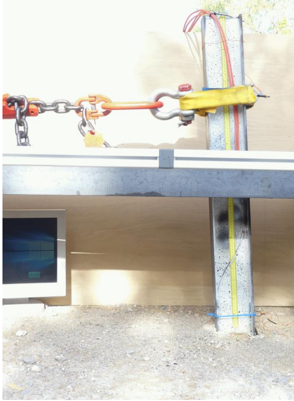
Fig. 3-26: Static test P01 sequential photos at 0%, 10%, 50% and 100% of the maximum force
