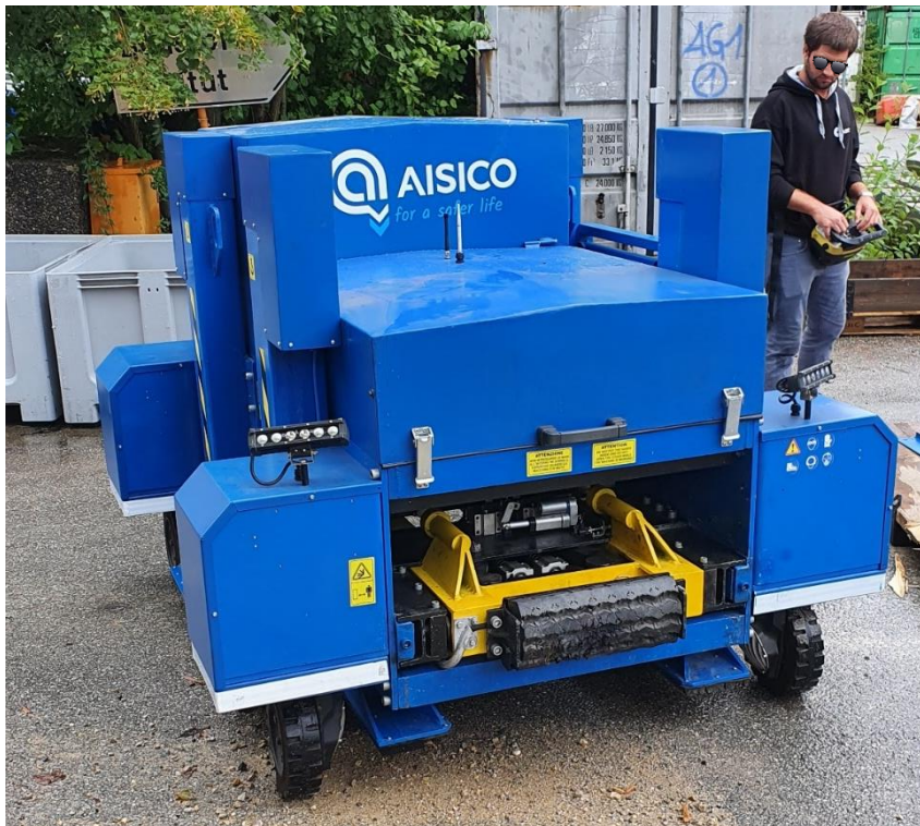
Fig. 3-36: Dynamic testing equipment THOR3 developed by AISICO srl.
