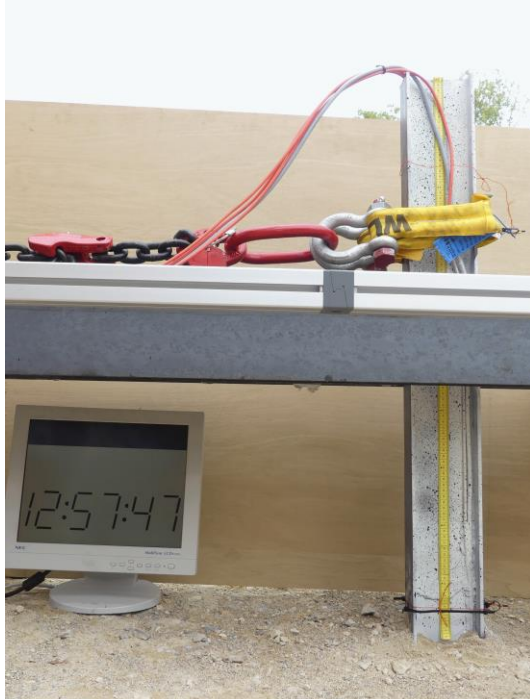
F=10% F max = 1.56 kN, u=9 mm
