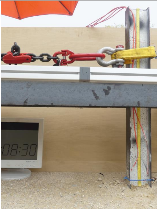
F=10% F max = 1.58 kN, u=5 mm
