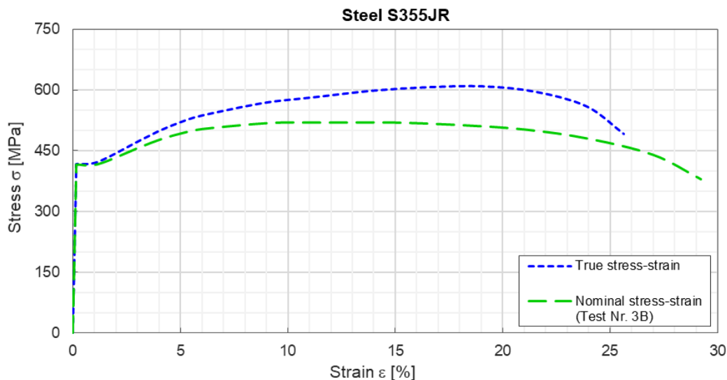
Fig. 5-8: Nominal versus true stress-strain values of the steel material applied for the post model
