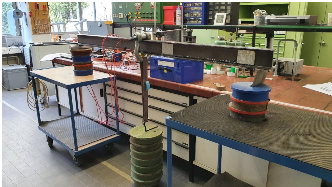
Fig. 3-23: Calibration of the installed strain gauges
