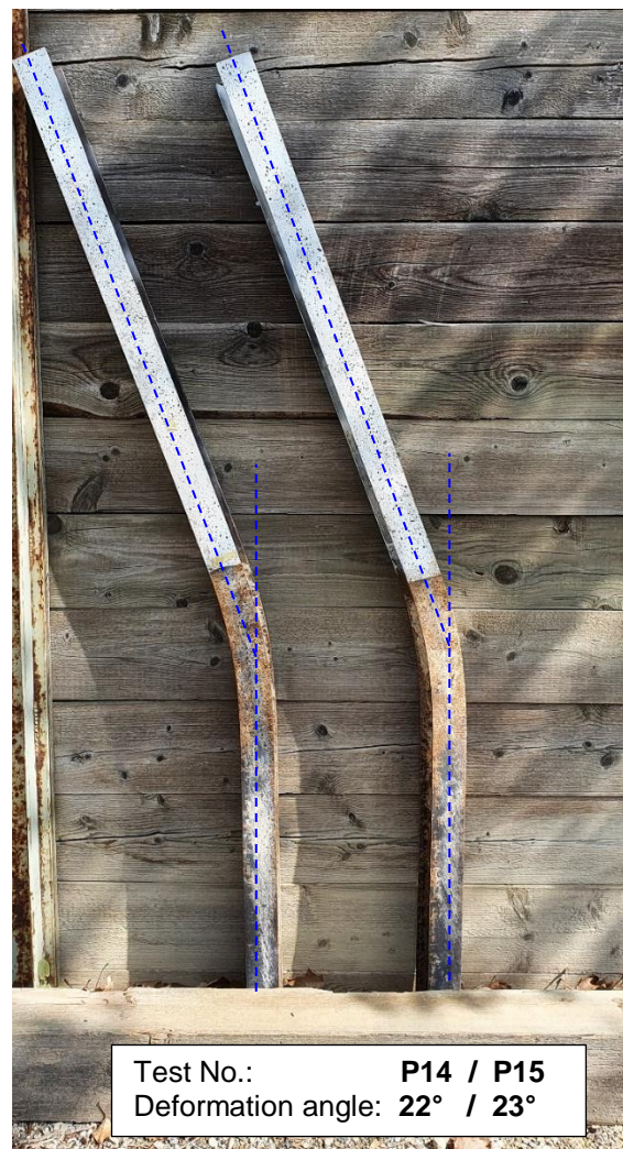
Fig. 3-31: The excavated posts tested in the weak axis P14 and P15 showing yielding of the steel post
