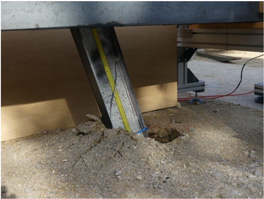
Fig. 3-27: Soil heave in the loading direction and formation of a gap behind the post
