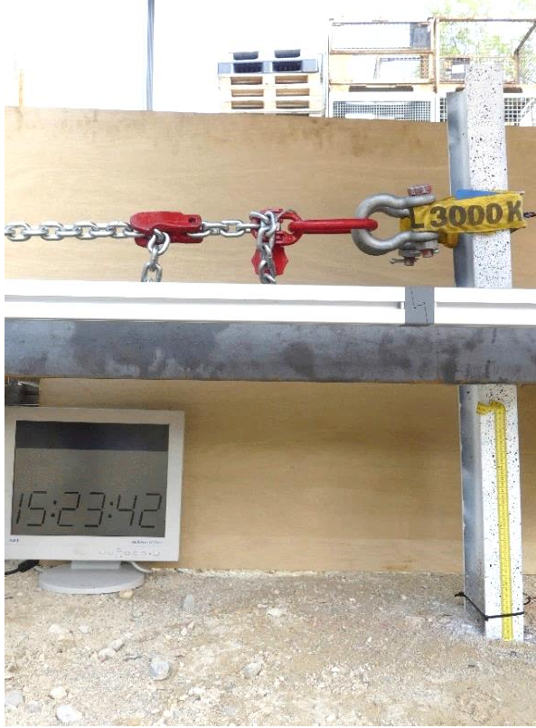
Fig. 3-30: Static test P14 sequential photos at 0%, 10%, 50% and 100% of the maximum force
