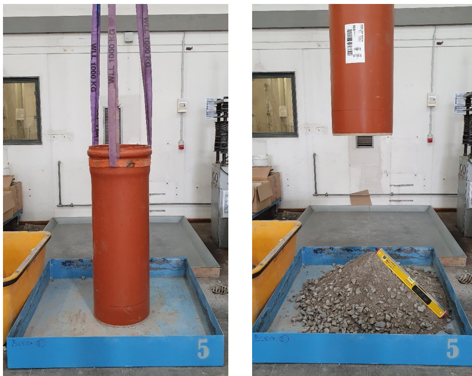
Fig. 4-8: Conduction of the large-scale angle of repose tests and formation of the soil heap
