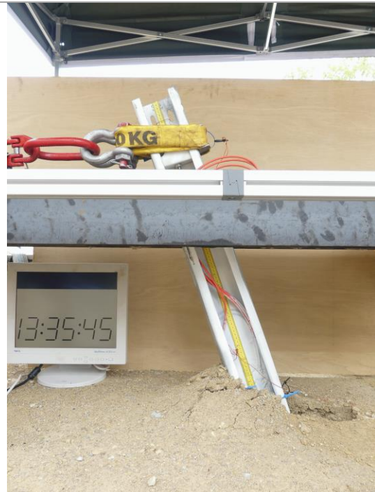
F=100% F max = 14.03 kN, u=416.4 mm
