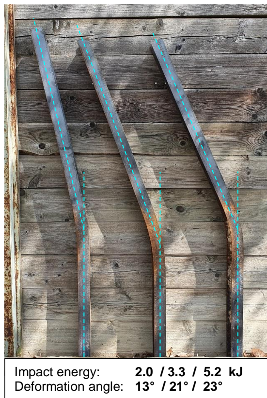
Fig. 3-53: The excavated IPE120 posts tested in the weak axis under different impact energy levels showing yielding of the steel post
