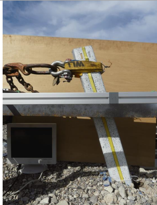
F=100% F max = 36.71 kN, u=303.8 mm
