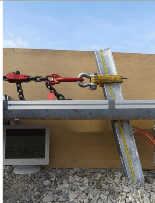
F=100% F max = 31.77 kN, u=251.7 mm
