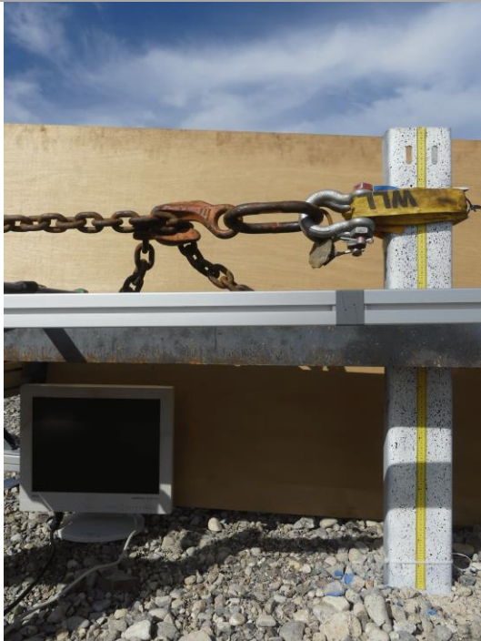
F=10% F max = 3.67 kN, u=8.6 mm
