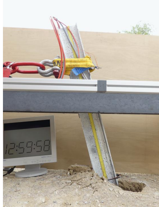
F=100% F max = 15.60 kN, u=349 mm
