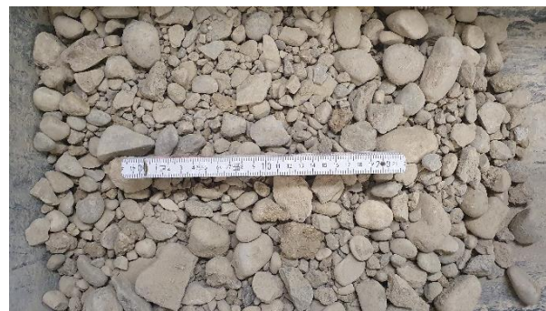
Fig. 3-3: Photos of the road shoulder materials selected for the experimental field tests
