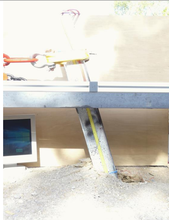
F=100% F max = 15.37 kN, u=340 mm
