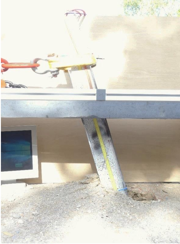
Fig. 3-26: Static test P01 sequential photos at 0%, 10%, 50% and 100% of the maximum force
