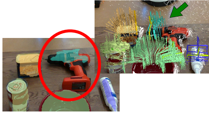
Figure 5.7: One advantage of our method is that it does not rely on an accurate segmentation of unknown objects. Here, successful grasp contacts are still found on the driller despite severe under-segmentation.
