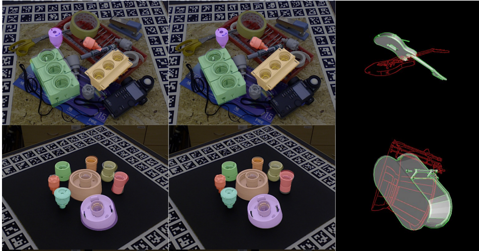
Figure 4.13: Left: Qualitative 6D Object Detection results of the RGB-based pipeline on T-LESS Primesense scenes. Only 18 of 30 objects are used to train the Multi-Path encoder; Middle: ICP-refined results; Right: Relative pose refinement of instances from the untrained categories guitar and bathtub. Red is the initial pose, green depicts the refined pose.
