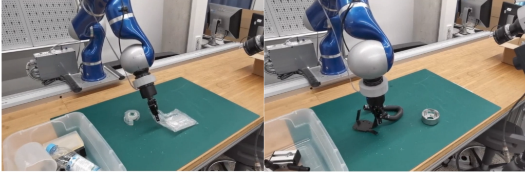
Figure 7.1: The use of stereo images and algorithms improves performance on transparent and black materials over ToF images.
