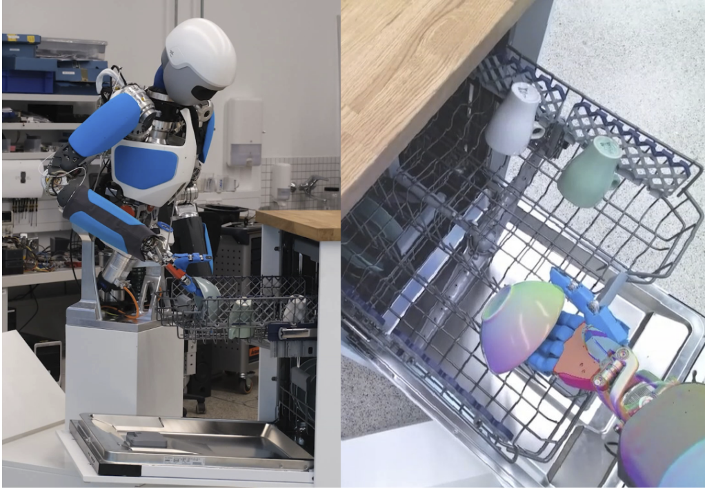
Figure 1.1: Humanoid robot David empties a dishwasher based on object detection [225], 6-DoF pose estimation [181] and refinement/tracking [214].
