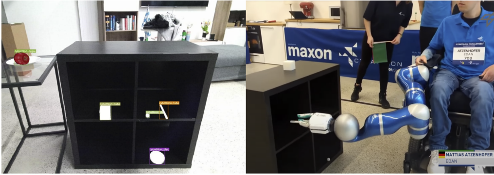
Figure 6.3: EDAN at CYBATHLON 2023. Left: 6-DoF object pose estimates from Yolov7 [225], AAEs [181] and ICG [214] of the challenge objects. Right: Shared-autonomy pick and place tasks during the CYBATHLON challenge. Matthias steers the arm towards the object and EDAN executes successful grasp using the estimated 6-DoF pose.
