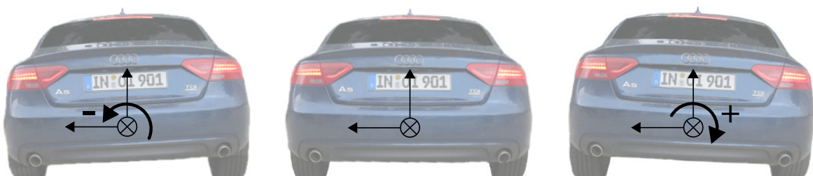
Figure 2.12: Positive (right) and negative (left) roll motions of the automated driving vehicle compared to the horizontal position (middle) taken from Cramer (2019) referring to Cramer and Klohr (2019)
