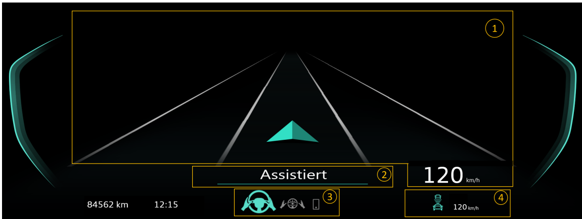
(a) Display in ASD including the four sections: (1) simulation, (2) description, (3) status, and (4) function
