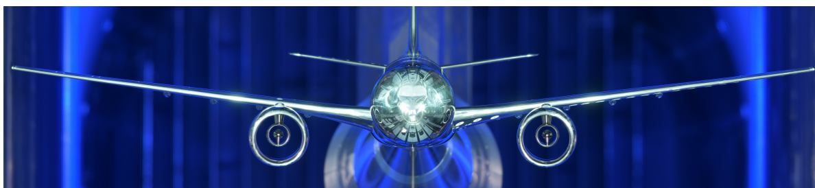
Figure 5.2: Front view of the Airbus XRF-1 wind tunnel model with UHBR engine nacelles installed (©Airbus/ETW).
