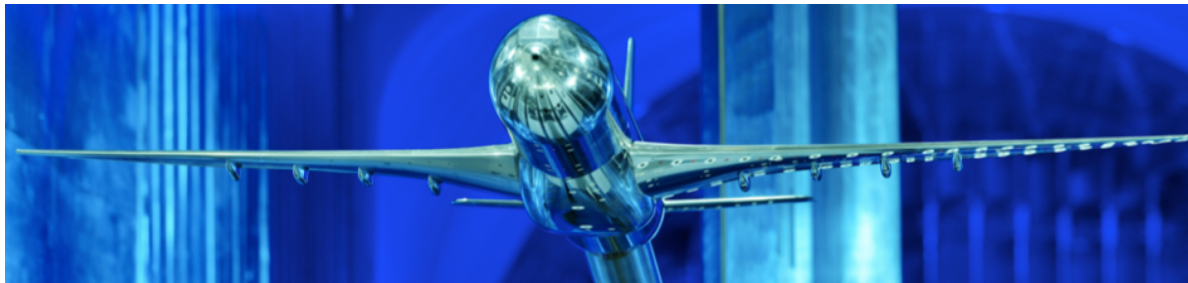
Figure 5.1: Front view of the Airbus XRF-1 wind tunnel model with clean wings (©Airbus/ETW).
