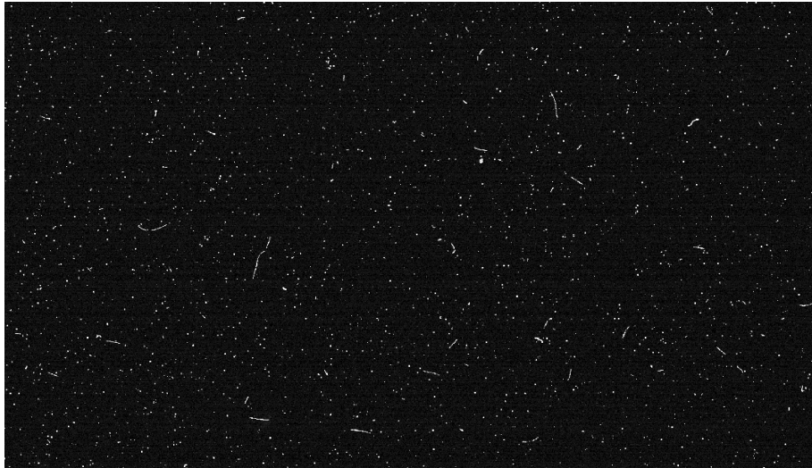
Figure 6.12: Section of an image acquired by an unmodified sensor. Numerous white streaks are visible across the frame with lengths varying between 10 and 70 \mu\text{m} . The most likely source for the white streaks are high energy ( > 60 \text{ keV} ) electrons resulting from the Compton scattering of the \gamma s produced from positron annihilation.
