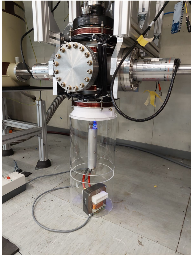
Figure 5.8: The isolation transformer and the 5 V power supply mounted to the underside of the sample chamber. Not shown in the photo, the high voltage cable providing the acceleration potential used to set the positron implantation energy.
