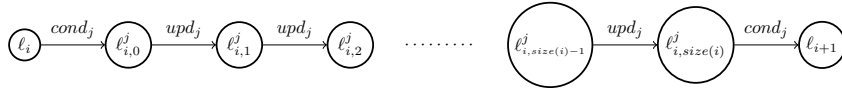
■ Figure 5 Third gadget, which guesses the partition. Here cond_j is the condition x_j \geq \sum_{l \neq j} c_l and upd_j is the update \bigwedge_{l \neq j} x_l++ .
