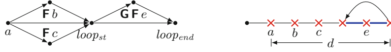
Fig. 4. The cut graph of a formula \mathbf{F}(a \wedge \mathbf{F}b \wedge \mathbf{F}c \wedge \mathbf{G}d \wedge \mathbf{G}Fe) (left) and one lasso shape for a chosen topological ordering a \leq \mathbf{F}b \leq \mathbf{F}c \leq \text{loop}_{st} \leq \mathbf{G}Fe \leq \text{loop}_{end} (right).
