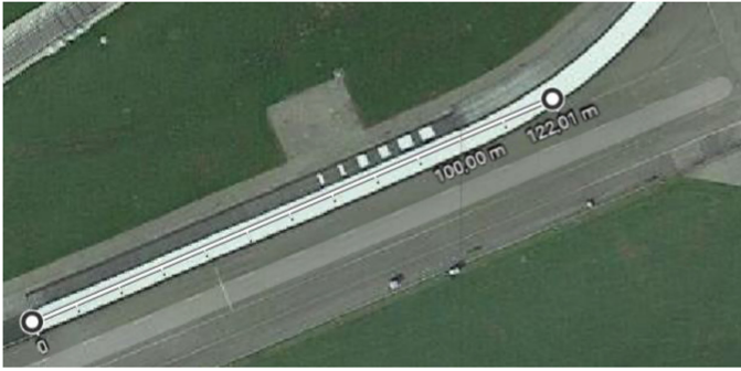
Fig. 9. Measurement in the proving ground. Track length of approximately 122 m. Surface covered by white tiles and filled with water [64].
