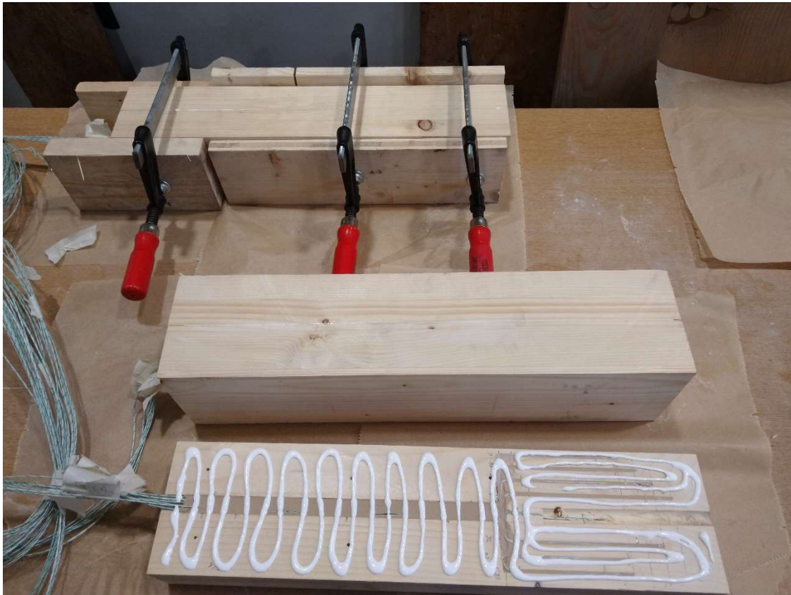
Figure 5: Inserting of thermocouples and Conlit in the reference specimen (top), Gluing of the two specimen halves of the reference specimen (bottom)
