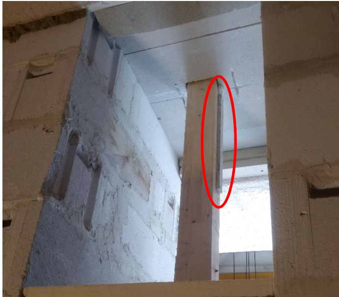
Figure 3: Protection and position of the sheathed thermocouple for the measurement of the rod temperature
