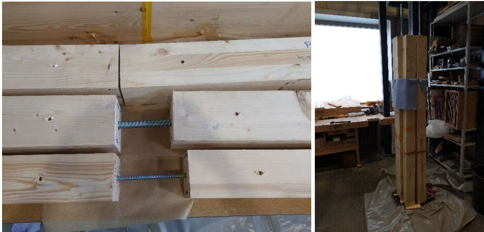
Figure 2. Inserting of the middle rod (left), Gluing process of the outer rods (right)
