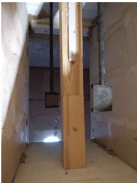
Figure 9: Positioning of thermo plates
