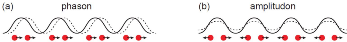
Figure 4.2.16.: Schematic explanation of the two vibrational modes in a linear chain of atoms interlaced with a charge density wave. The depicted phason changes the dipole moment and is consequently infrared active, whereas the amplitudon describes a Raman active oscillation. The latter can be used to investigate the properties of the electron collective via Raman spectroscopy. Picture adapted from [67].
