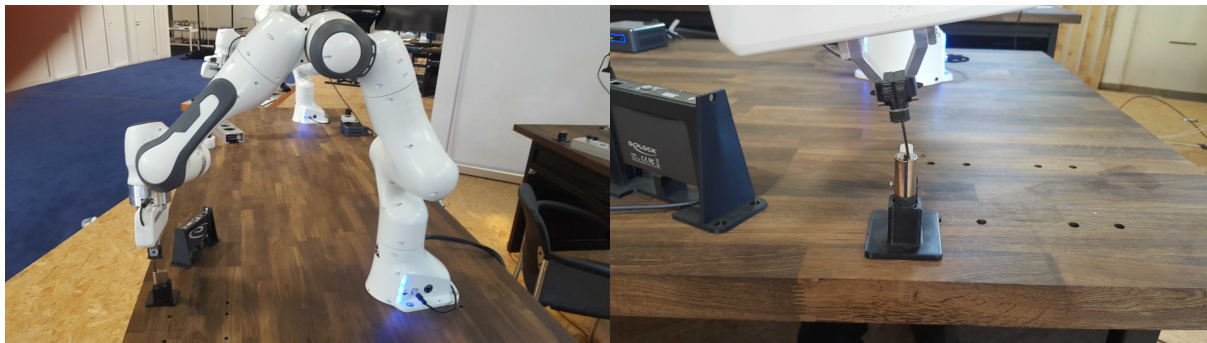
Figure 4.5: Experiment setup consisting of a robot arm and a key/lock combination
