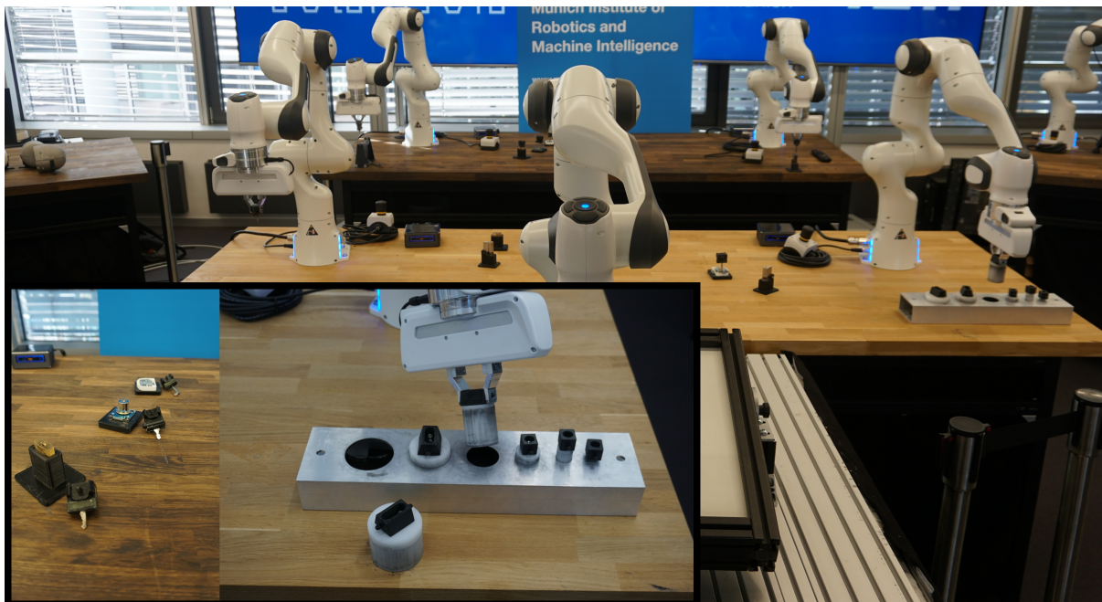
Figure 4.8: The analyzed reference tasks consist of six cylinders with increasing diameters and three different common household keys (bottom left). Five robots were used in total for the experiment.
