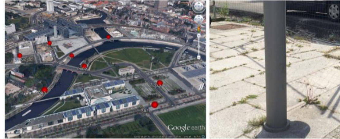
Reference points (red dots) in the optical image of Berlin. All of the candidates are assumed base of lamp posts*
