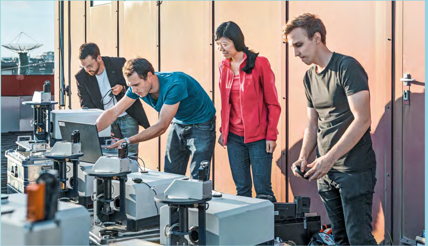
Side-by-side measurements: Jia Chen and her colleagues calibrate their sensors before a six-week series of carbon dioxide, methane, carbon monoxide and nitrogen oxide measurements in Munich in autumn 2017. The results will contribute to a larger international study. Left to right: Ralph Kleinschek (German Aerospace Center – DLR), Florian Dietrich, Jia Chen, Michael Wedrat (TUM).
