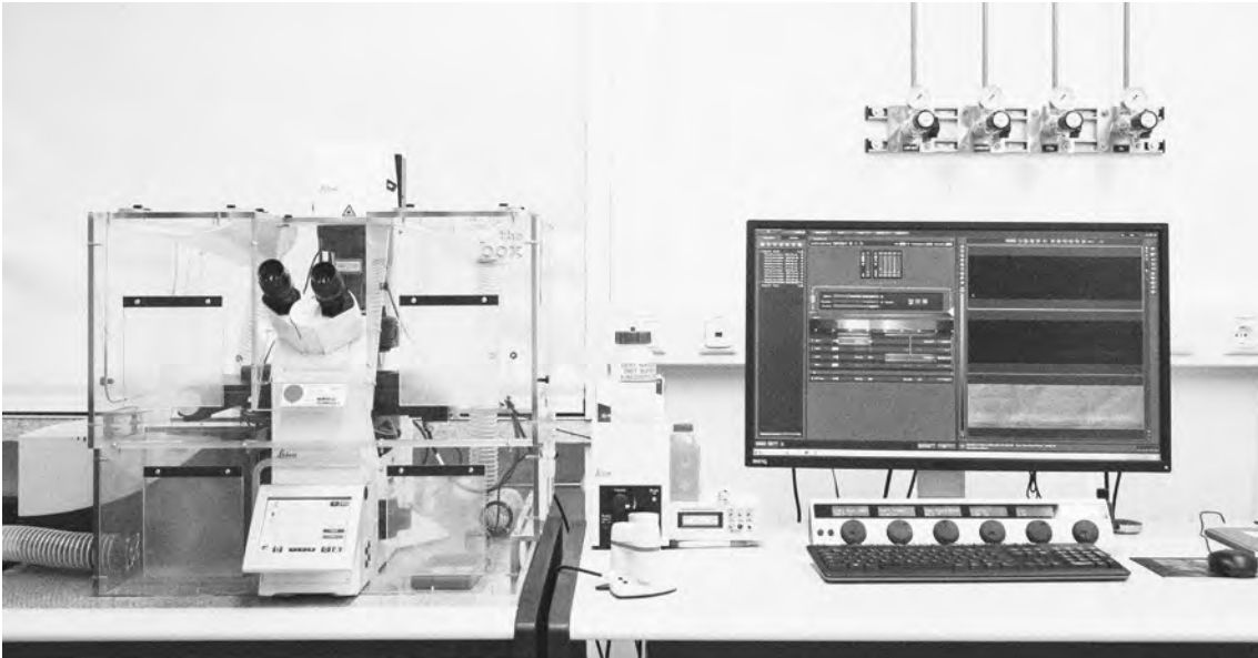
Confocal laser scanning microscope: Tim Czopka and his team investigate interactions between neurons and glia using a combination of high resolution microscopy methods, genetics and modern data analysis.
