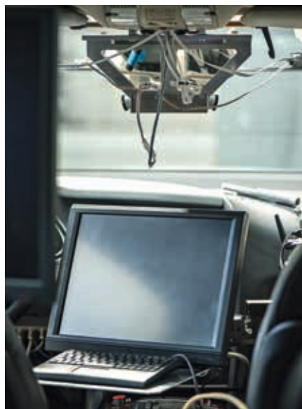
Camera systems record the front and side view from the cockpit. All images are transmitted via mobile communication to the operator, who controls the steering wheel and pedals.
