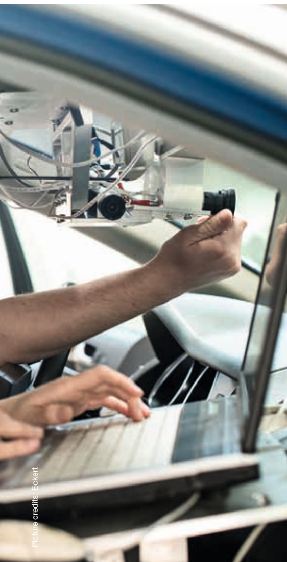
Camera systems record the front and side view from the cockpit. All images are transmitted via mobile communication to the operator, who controls the steering wheel and pedals.
