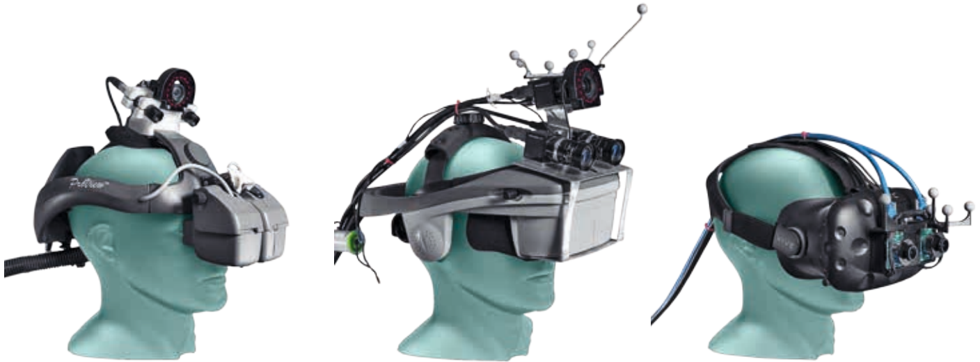
This RAMP Head Mounted Display (HMD) system was developed at Siemens Corporate Research at the end of 1990s.
