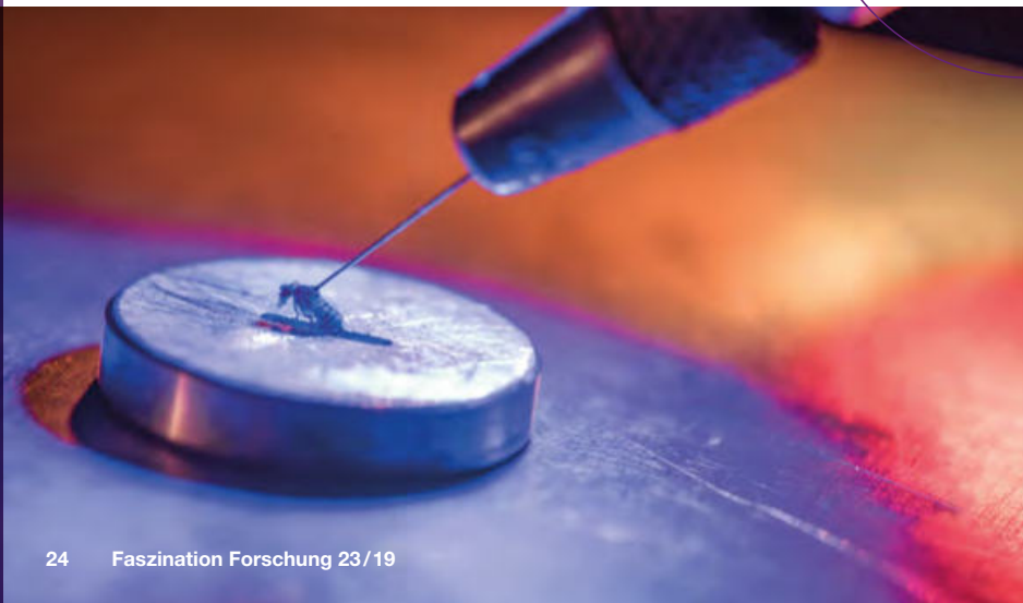
The team anesthetizes the flies with cold or CO 2 and uses tweezers and micromanipulators to position them under the microscope. They are glued into place with UV-cured dental adhesive, which hardens extremely fast.
