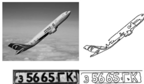
Figure 2.9: An example of an edge detection algorithm operation. The figure is taken from [Kho12].
