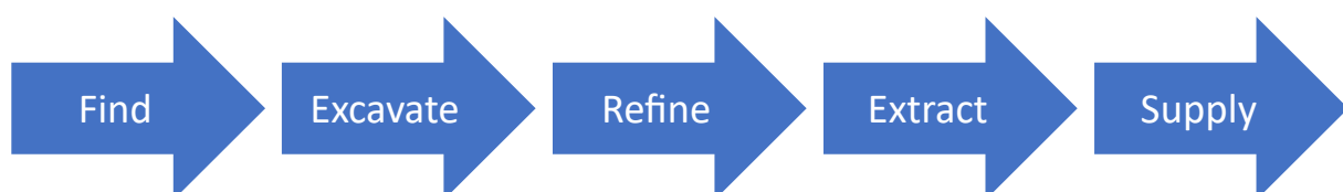
Figure 1-2: Simplified ISRU value chain (ISECG 2021)
