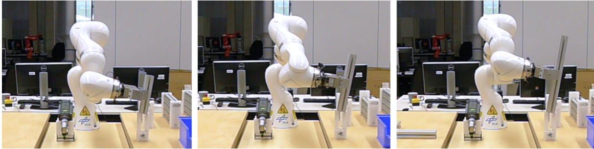
Figure 4: Insertion of aluminum profiles of varying length into an assembly fixture. The execution should adapt autonomously to the individual constraints of the tasks without generating manual programming effort.
