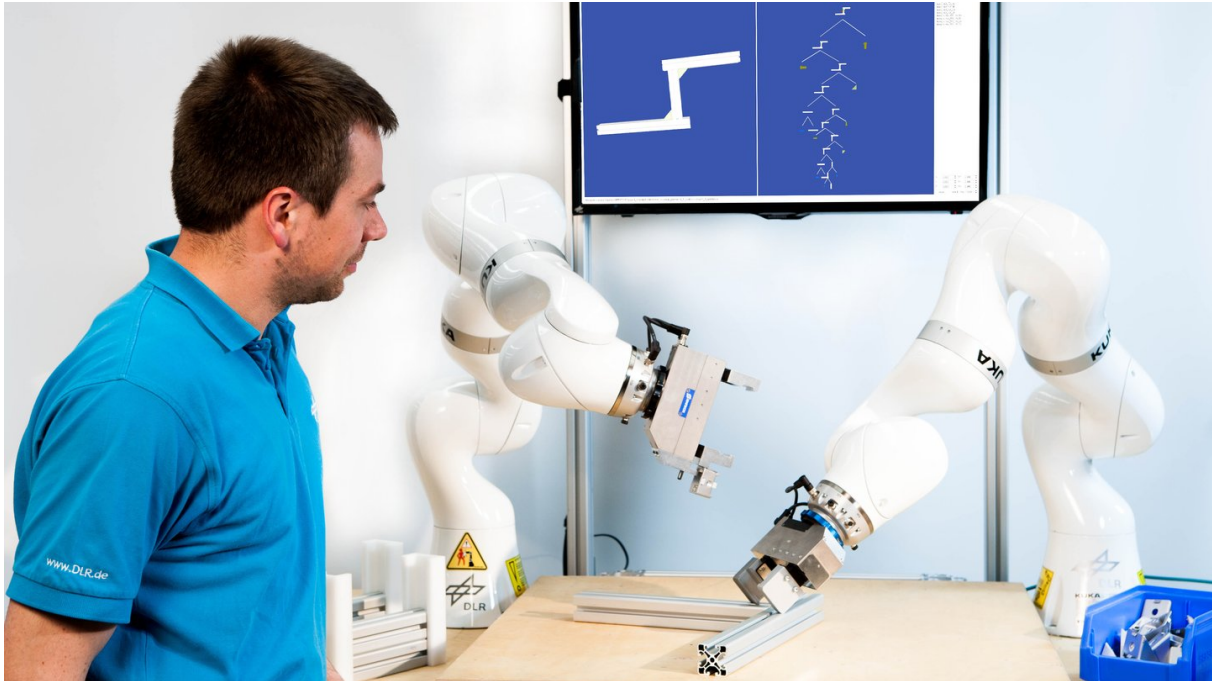
Figure 18: Assembly of aluminum profile structures with a flexible robotic assembly system. Source: Courtesy of DLR, CC-BY 3.0, also appearing in Publication 4 (Fig. 1)
