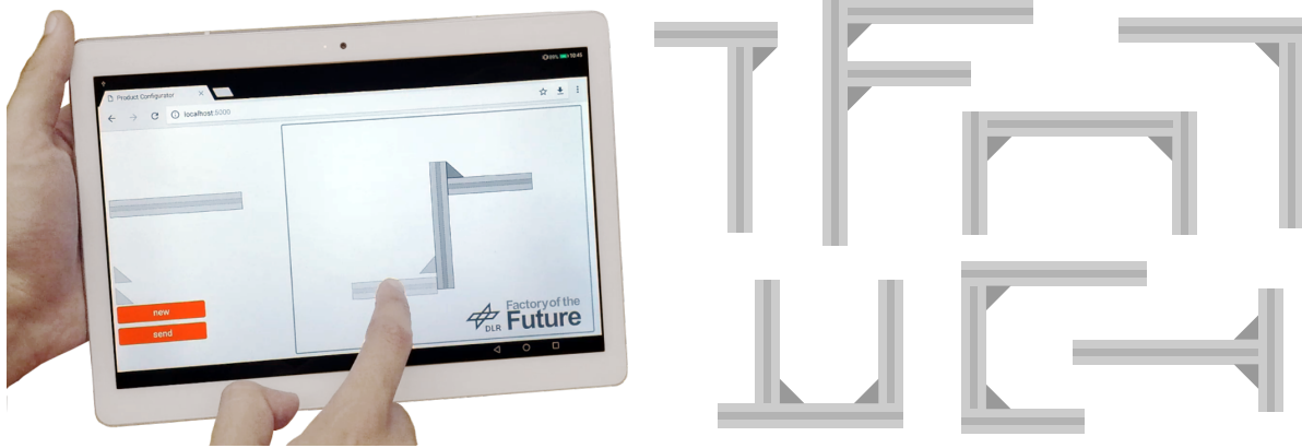
Figure 2: By using a dedicated product configurator with an intuitive interface, customers are able to design individual products without considering the required production processes. Here, the products are aluminum structures composed of parts from a modular construction set. Source: Courtesy of DLR (left)
