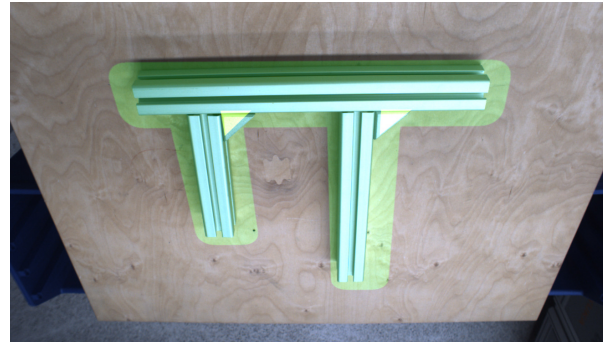
Figure 2: Recognition of the desired assembly by the camera above the workbench, and visual feedback to the user highlighting the detected structure (in green).
