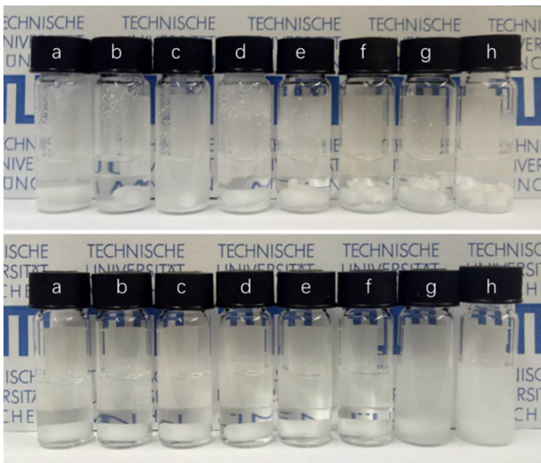
Figure 6.2: Photographs of the sol-gel solutions prepared with THF (a to d) and 1,4-dioxane (e to h). The picture at the top clearly shows the white crystalline solids by adding SnCl 4 in to the cycloether solvent, and the picture below is the corresponding sol-gel solution after adding HCl catalyst. The HCl content added in to the sol-gel solution is 50 μl(a, e), 100 μl(b, f), 150 μl (c, g), and 200 μl(d, h), respectively. Reproduced from Ref [111] with permission from JOHN WILEY AND SONS, Copyright 2020.
