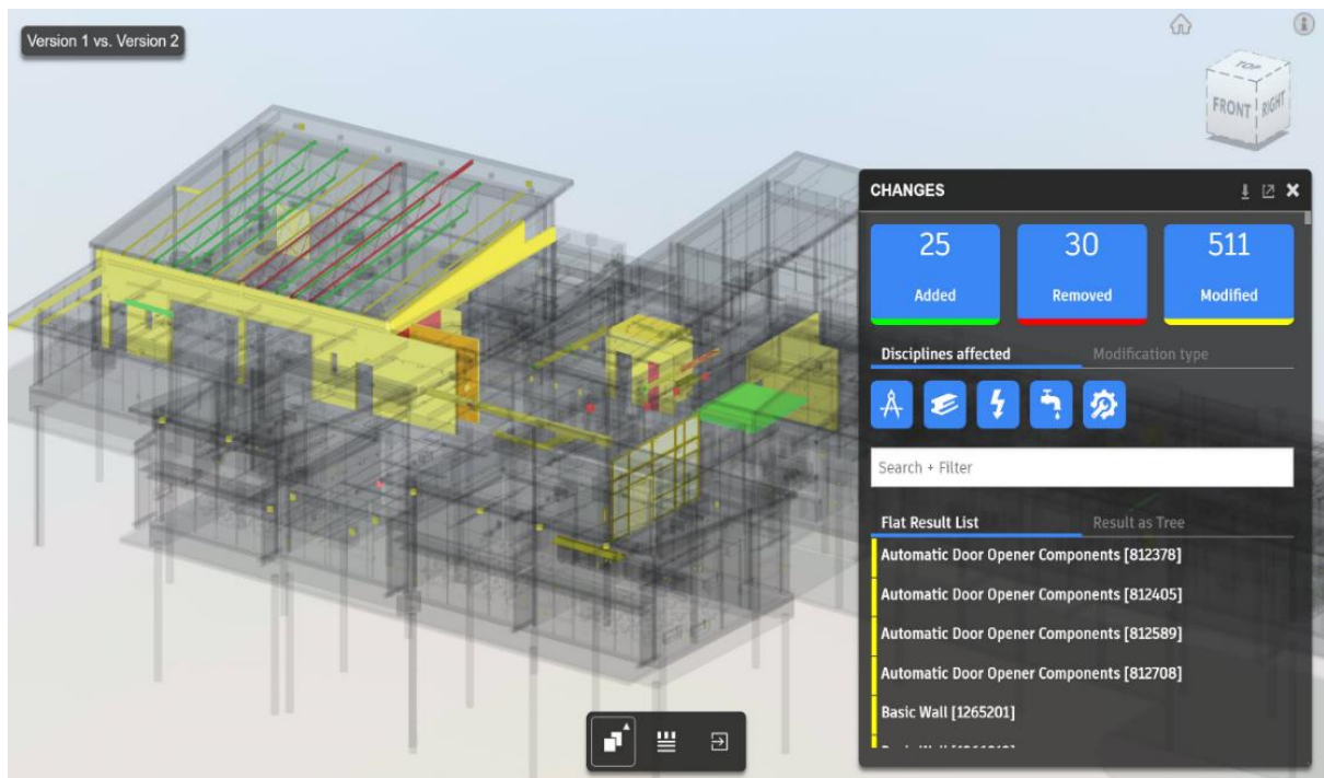
Figure 22 - Output from comparing two model versions in BIM 360 (Autodesk).
