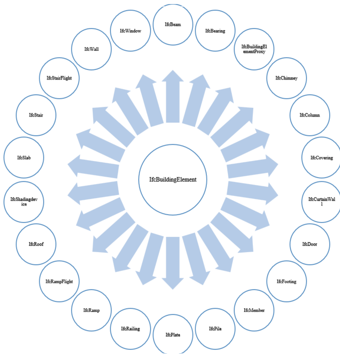
Figure 10 - Classes derived from IfcBuildingElement superclass.
