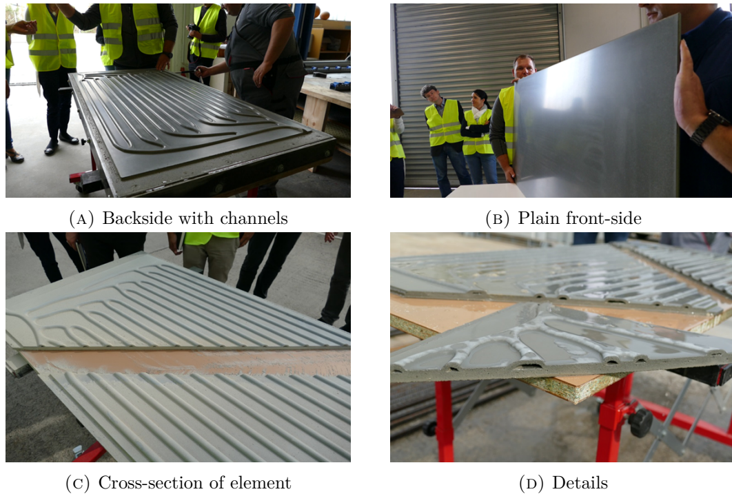
FIGURE 4.2.7. TABSOLAR ® element with channels
