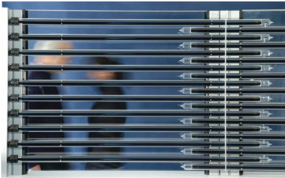
FIGURE 2.2.5. Mock-up of semitransparent BIST element [166]
