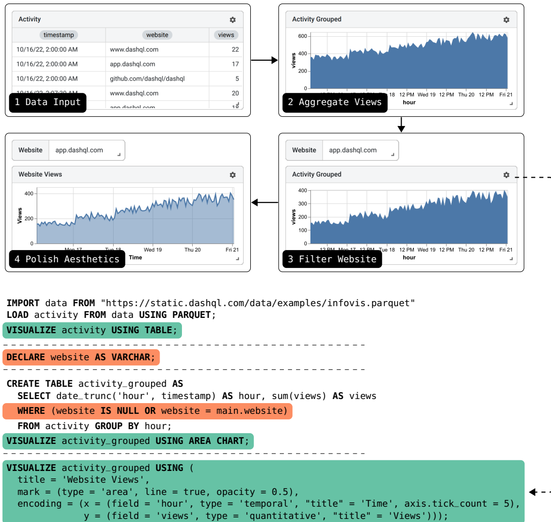
Figure 10: Authoring an example analysis workflow with DashQL. The workflow explores website activity data in four steps. The steps are labeled with ① to ④ and associate textual changes in the script with adjusted visual output. Visualization statements are colored in green, the input statement and the corresponding predicate in orange.
