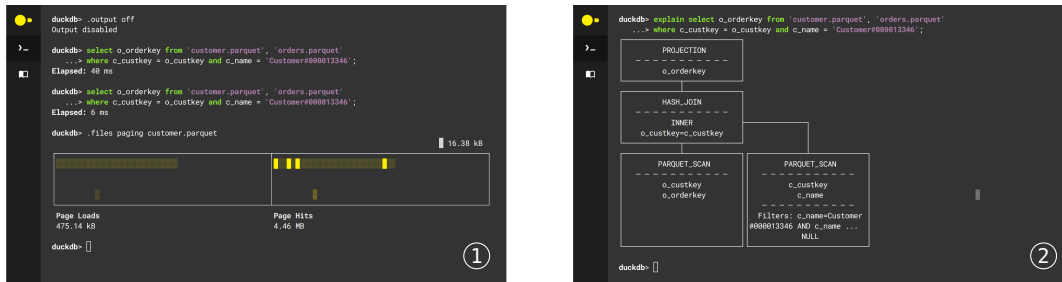
Figure 42: A shell that runs entirely in the browser and evaluates SQL queries using DuckDB-Wasm. The figure shows a query joining two parquet files with the relations orders and customer of the TPC-H benchmark at scale factor 0.1. ① lists the query results and page accesses, ② shows the query plan.
