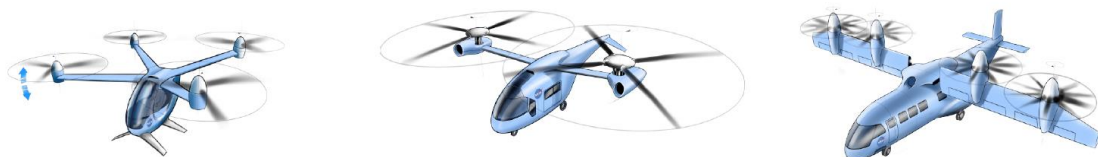
Figure 3.4: Exemplary NASA Concept Vehicles: Quadrotor, Side-by-Side Helicopter, and Tilt-Wing Aircraft Concept [7]
