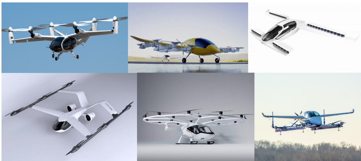
Figure 1.1: Electric VTOL Aircraft. Top row: Joby S4, Kitty Hawk Cora, Lilium Jet. Bottom row: Voloconnect, Volocity, Aurora PAV (Sources: Company sites and evtol.news)
