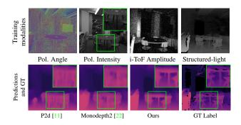
Figure 1. Top row: polarisation input signal (Pol.) visualised as Angle and Intensity. Additionally; Time-of-Flight Amplitude (i-ToF) and structured-light sensor co-modalities, exploitable during training. Bottom row: monocular depth estimation, using the Pol. input. Uni-modal model training of p2d [11] and the monodepth2 architecture [22], compared with cross-modal training (Ours).
