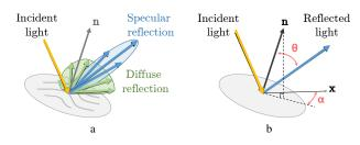
Figure S1. (a) differing types of reflected light and (b) the link between a surface normal **n**, its viewing angle  $\theta$  and its azimuth angle  $\alpha$  (right).
