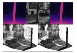
Figure 4. Effect of the *Displacement Fields* (DF). Left top (bottom): predicted depth (point cloud) without DF. Center top: polarisation intensity. Right top (bottom): predicted depth (point cloud) with DF. Flying pixels, visible in 3D, are clearly reduced.
