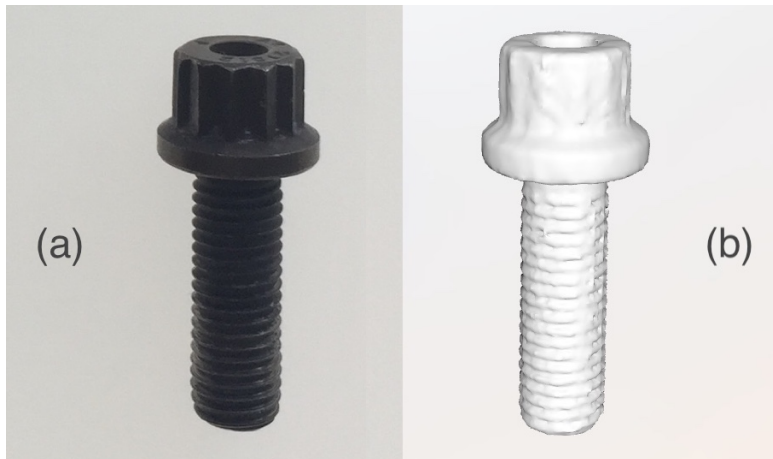
Figure 7.1: (b) is a 3D model of the small part (a) created by 3D scanning. The 3D scanner is unable to accurately capture fine details like the small part threads as shown in (b). The 3D model is rendered without texture for clarity.
