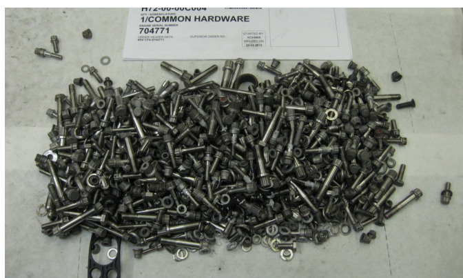
Figure 1.1: Small parts that were taken apart during an aircraft engine overhaul, and have to be sorted for reassembling.
