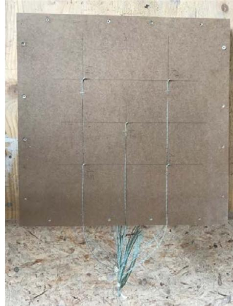
**Abbildung A.16.7-4: PK 2 Einbau TE in Mess-ebene 1**
