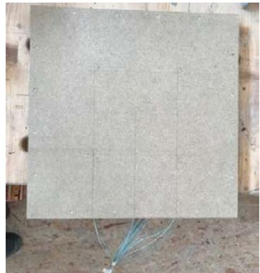
**Abbildung A.17.7-4: PK 4 Einbau TE in Mess-ebene 1**
