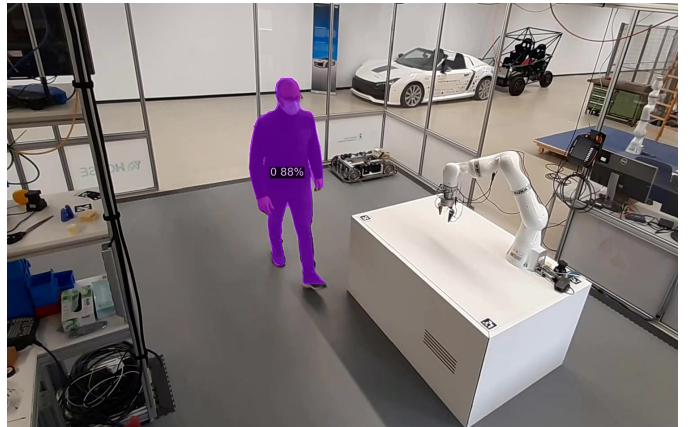
Fig. 5: Qualitative evaluation of S+R 1000* -BlendMask on a scene containing a robotic workcell with a Kuka LBR Iiwa and a human entering the robot's workspace.
