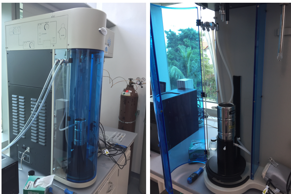
(a) The modified sidewall seen from the outside (clear part). Tubes lead to the Julabo thermostat. The door can now be fully closed. (b) The interior with thin, flexible tubes connected to the Dewar. This allows unrestricted up- and downward motion without obstruction.
