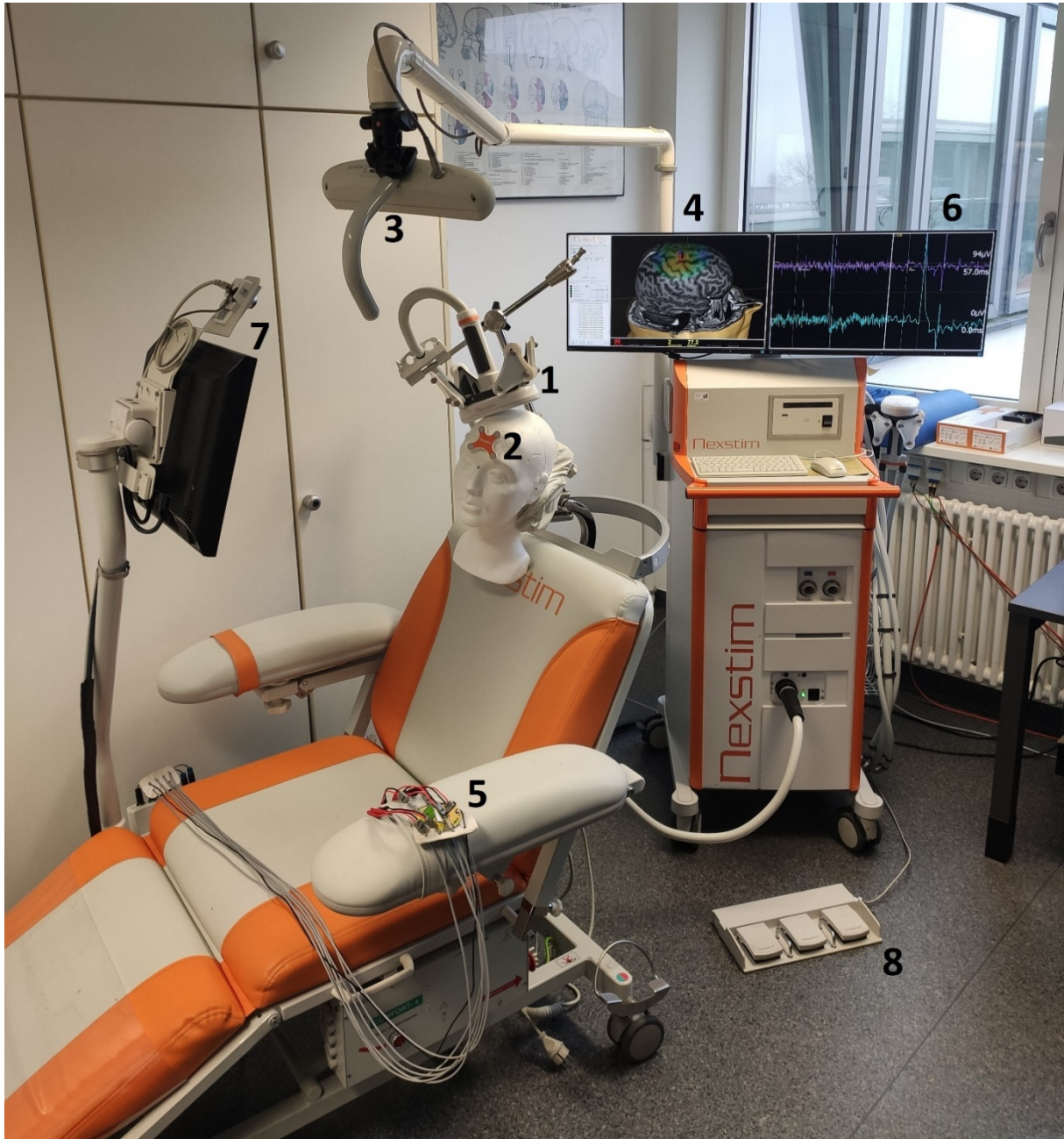
Figure 6 – System setup. Figure 6 displays a typical navigated transcranial magnetic stimulation setup. 1) Stimulation coil; 2) Model head with headtracker (orange); 3) Tracking camera; 4) Navigation display; 5) Electromyography (EMG) cables; 6) EMG display; 7) Monitor and videocamera; 8) Trigger pedals.
