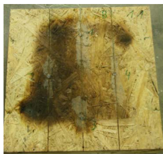
2 x 18 mm Typ DF T_{\max} = 250 \text{ }^{\circ}\text{C} \varnothing T = 225 \text{ }^{\circ}\text{C} 90 min ETK
