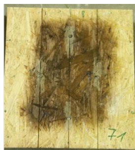
2 x 18 mm Typ DF T_{\max} = 250 \text{ }^{\circ}\text{C} \varnothing T = 240 \text{ }^{\circ}\text{C} Naturbrand_1
