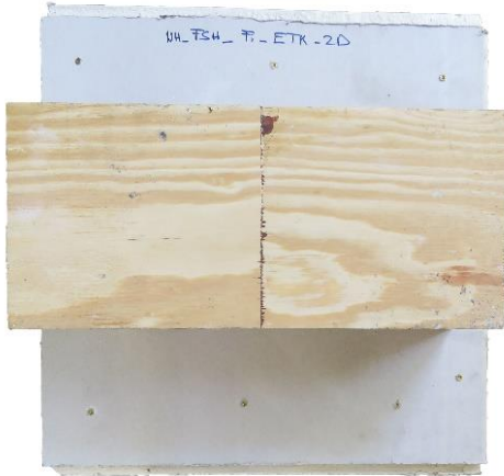
NH_FSH_Fi_ETK_2D Versuchskörper, unbeanspruch
