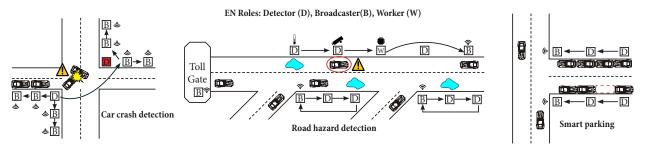
(a) Car crashes on the road can be detected with the support of cameras. The detector node will pass the information to all nearby broadcasters to send a notification to as many vehicles as possible. In this case, a redundant detector node is deployed to counter possible node failures.
