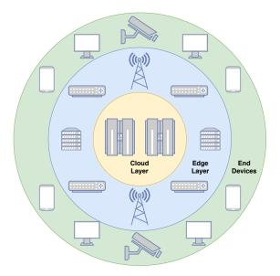
Figure 2.1: Edge-cloud layers structure.
