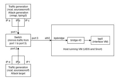
Figure 3.4: Setup for live traffic.
