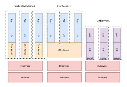
Figure 4.2: Comparison of different virtualization technologies.
