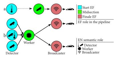
Figure 4.13: Pipelines' execution graphs based on ENs capabilities and EFs roles.
