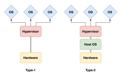
Figure 4.1: Comparison between Type-1 and Type-2 hypervisors.
