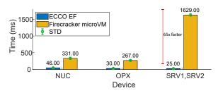
Fig. 5: Average ECCO EF vs. Firecracker microVM boot-up time and standard deviation (STD).
