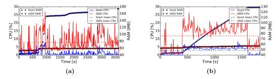
Figure 3.6: UIDS vs. Snort (CICIDS2017, RPI) — Port scans (a) and DoS (b).
