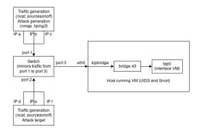
Fig. 3. Setup for live traffic.
