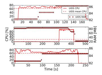
Fig. 10. UIDS stress-test (LAP) — Saturated 1Gbps link (top). Background traffic plus attacks (middle). 1Gbps, 5000 concurrent TCP connections (bottom).
