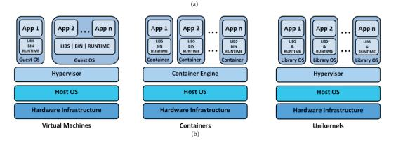
Figure 3: LV techniques comparison. (a) Quantitative analysis; (b) Core architectural differences
