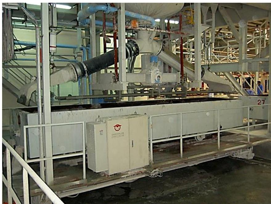
**Figure 2.1** Casting the AAC mixture into the molds. This figure is reprinted with permission from Schober [72].
