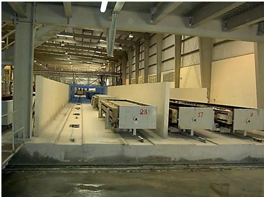
**Figure 2.2** Storing the AAC mixture. This figure is reprinted with permission from Schober [72].
