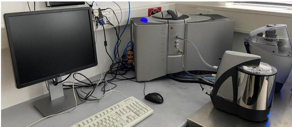
**Figure 3.16** Malvern Mastersizer 3000, used for determination of particle size for powders.
