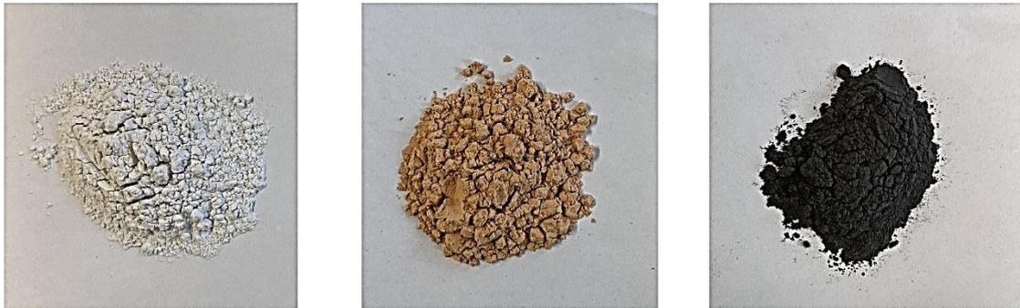
**Figure 3.1** Silica materials used in this study. From left to right, quartz sand, C-DE, and RHA.
