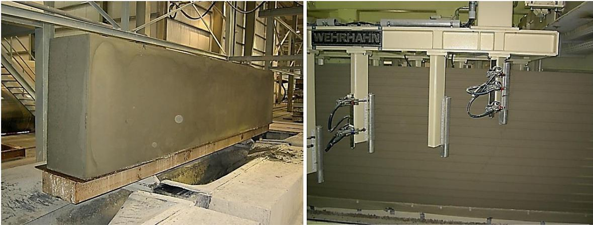
**Figure 2.3** Demolding (left) and cutting (right) the AAC green cake. This figure is reprinted with permission from Schober [72].
