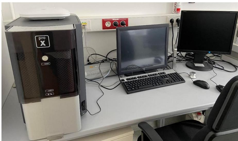
**Figure 3.14** Phenom Pro X, used to examine the microstructure of samples.
