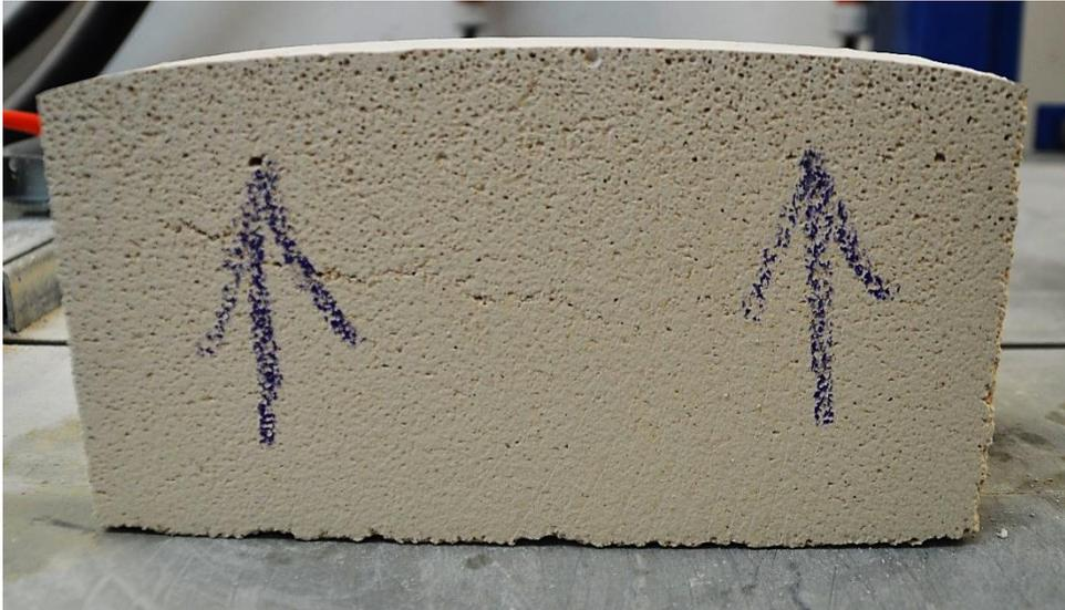
**Figure 3.11** Expansion crack which was observed in the samples.
