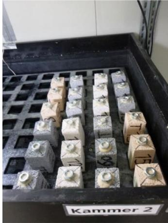
**Figure 9** Conditioning AAC prisms in water with a temperature of  $20 \pm 2$  °C for 72 h.
