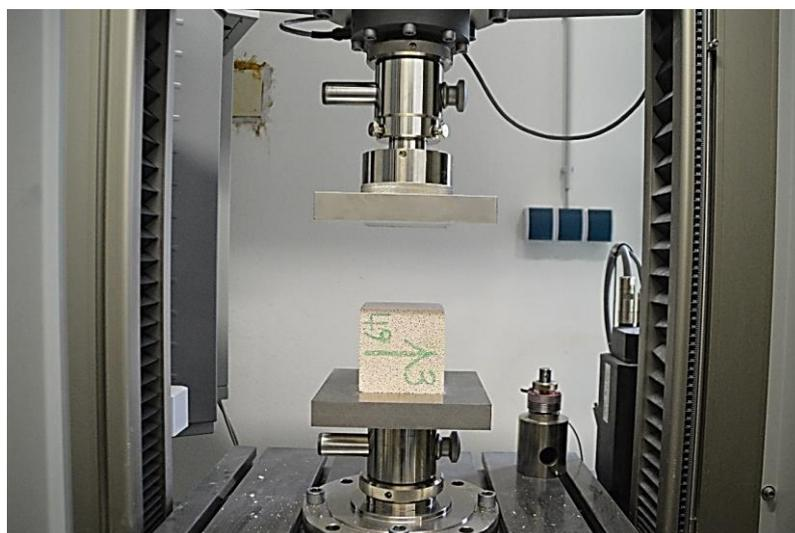
**Figure 3.12** Measuring the compressive strength with Zwick Roell Z 100.
