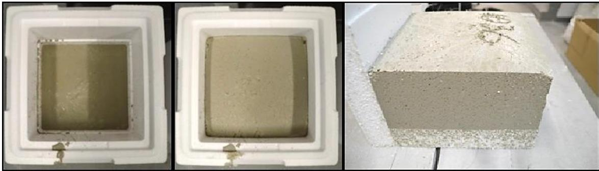
**Figure 3.8** From left to right, molding, rising to the final volume, and demolding.
