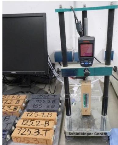
**Figure 10** First measurements of length ( $L_{c0}$ ).
