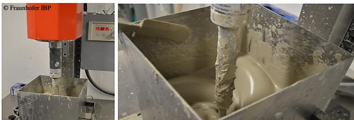
**Figure 3.7** The mixing process. This figure is reprinted from Fraunhofer IBP archive.
