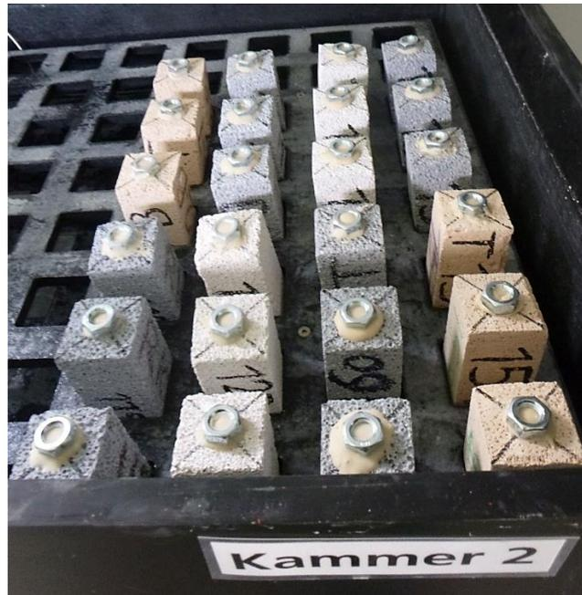
**Figure 3.18** Conditioning AAC prisms in water with a temperature of  $20 \pm 2$  °C for 72 h.
