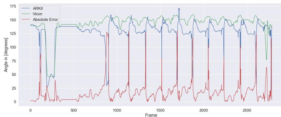
**Figure 11.** Left elbow angle of one of the subjects in the Single Leg Deadlift exercise, which shows several unexpected spikes during the execution. The spikes originate from ARKit incorrectly detecting the joint's position, most probably because of bad visibility of the elbow joint during the exercise.
