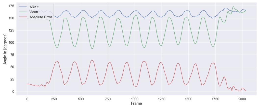
**Figure 7.** Left hip angle of one of the subjects in the Side Squat exercise in degrees. The plot shows that while the motion pattern is visible in both recordings, ARKit exposes a reduced amplitude and a shift on the  $y$ -axis.
