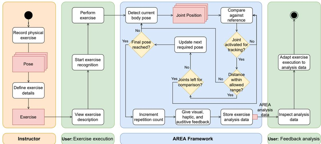
**Figure 2.5:** UML activity diagram representing the flow of events of the AREA algorithm. The diagram includes activities performed by the instructor to record a new exercise, the user by performing an exercise and analyzing their feedback, and the AREA framework recognizing and counting valid exercise repetitions.
