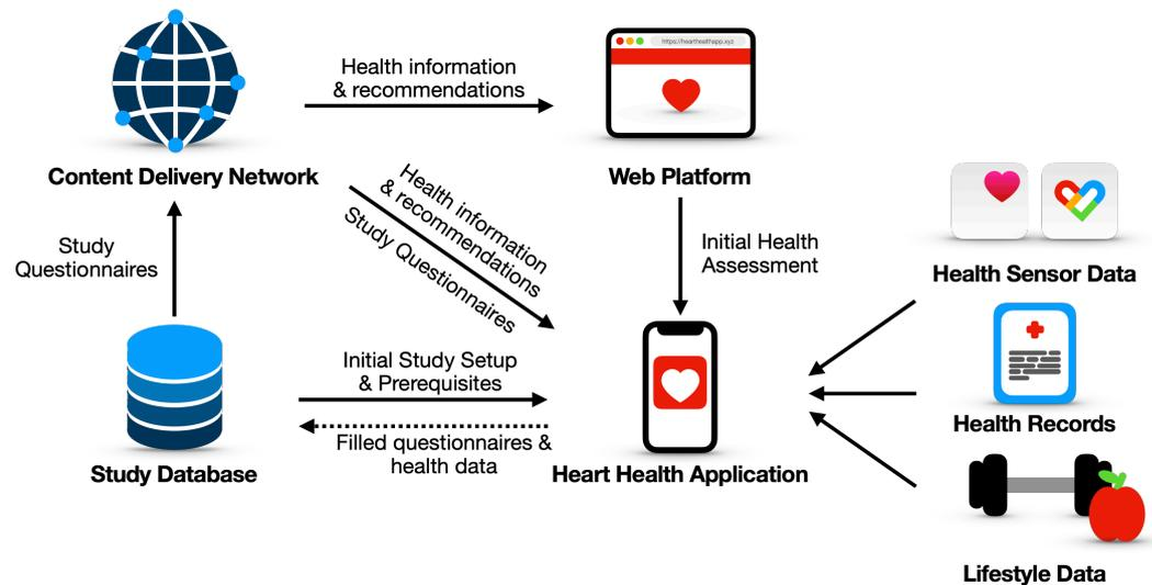
**Figure 2.7:** Overview of the data flow of the Heart Health Application, an example of how to perform scientific data collection on sensitive data such as health data.
