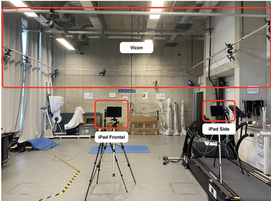
**Figure 2.3:** Camera setup of laboratory experiment B. The 14 *Vicon* infrared cameras are positioned around the subject close to the ceiling of the laboratory. Two iPads are positioned frontally facing the subject and in a  $30^\circ$  angle.
