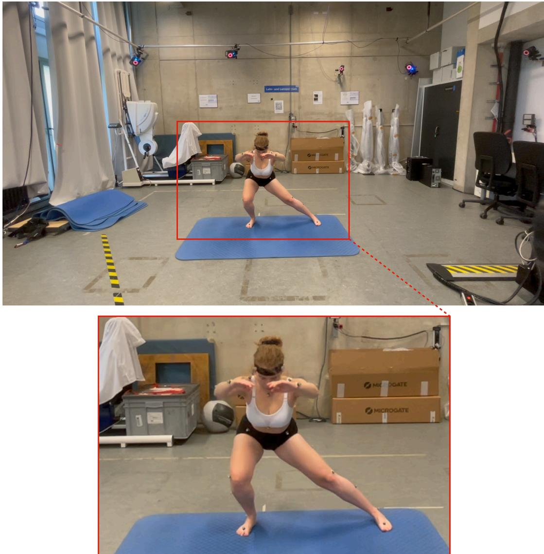
**Figure 3.1:** Woman being recorded by the *Vicon* system with reflective markers attached to her body. Infrared cameras are placed around the subject to capture the markers.
