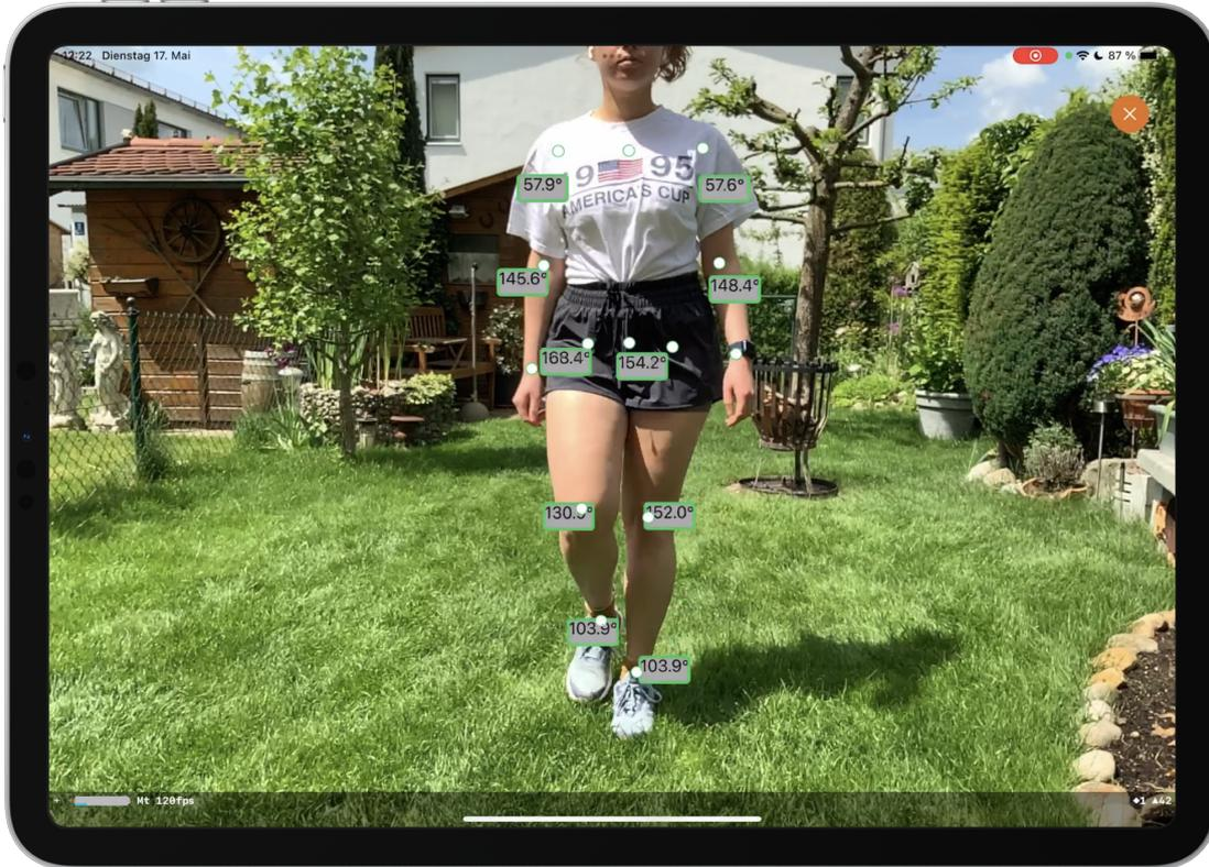
**Figure 3.2:** Woman being recorded by the *ARKit* system running on an iPad. The joints are detected by the camera and visualized on the screen including the detected joint angle in degrees.
