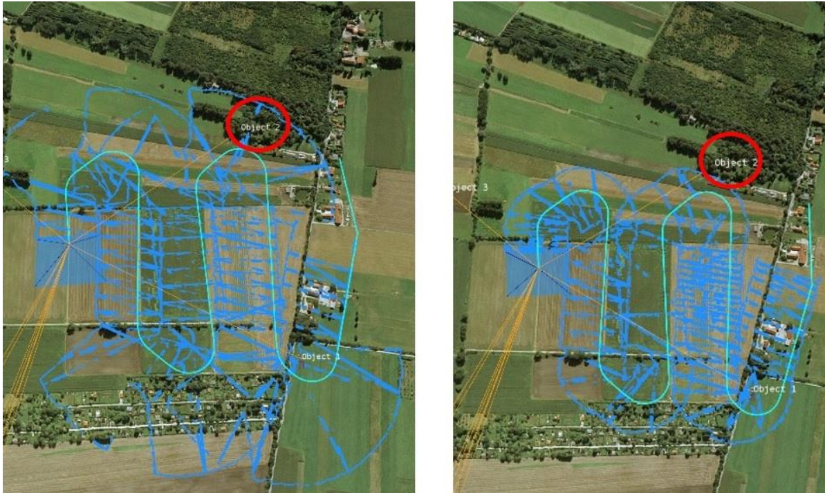
Figure 3.13: Sensor on board without gimbal (left) and with gimbal (right) (Fokina et al. 2018c)
