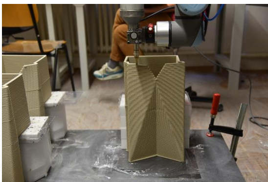
Figure 35: Documentation of 3D printing of the climate performative tile
