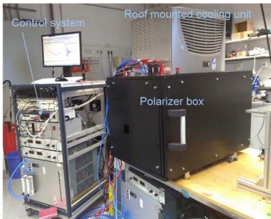
**Figure 2.** The polarizer box with roof mounted cooling unit and the control system
