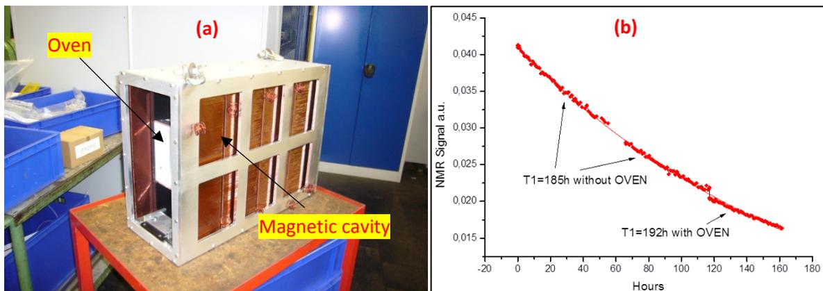
**Figure 3.** *a- The magnetic cavity with oven and  $^3\text{He}$  cell inside. b-  $^3\text{He}$  cell relaxation time. Measured  $^3\text{He}$  relaxation time of 185 hours for 3 bar  $^3\text{He}$  cell placed inside the magnetic cavity. Subtraction of the cells self-relaxation time yields a cell averaged equivalent gradient of  $5 \times 10^{-4} \text{ cm}^{-1}$ .*
