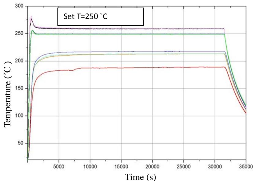
**Figure 5.** Test of the oven temperature stability, the different colors represent the readout from different sensors mounted in the oven. The cell reaches a stable temperature after  $\sim 2000$  s and remains then stable for the rest of the test.
