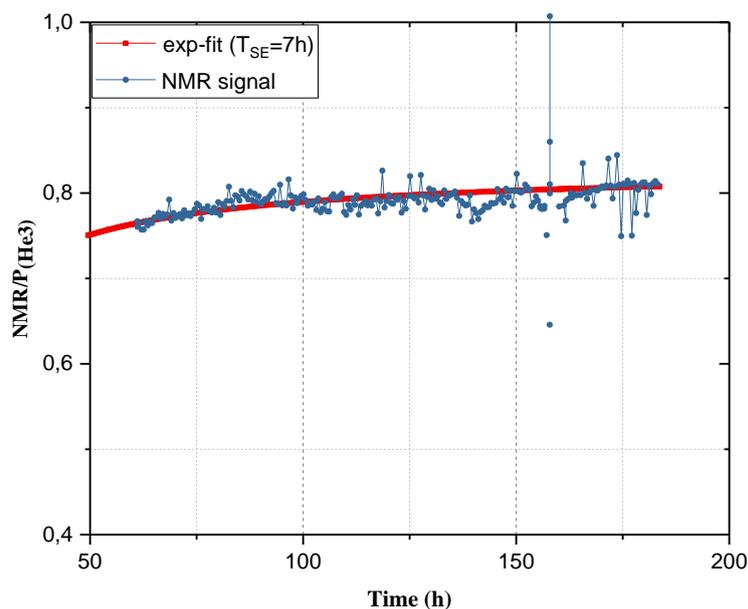
**Figure 7.** The  $^3\text{He}$  polarization as function of time obtained during on-beam test at POLI
