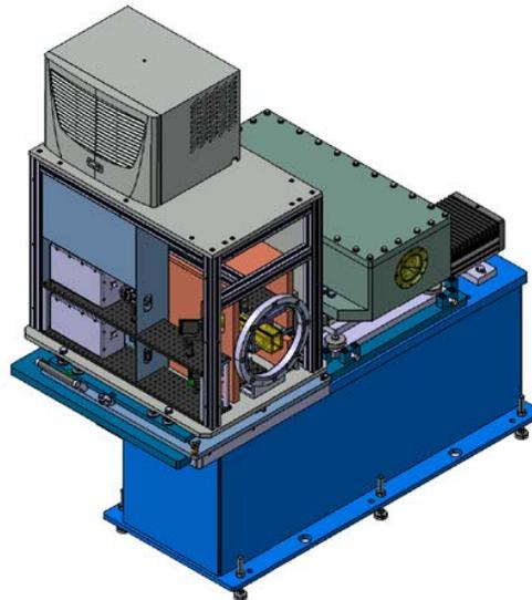
*Figure 1. CAD model of the guide changer with one stage for the neutron guide and one stage for the SEOP polarizer box including the oven, the laser system, and a chiller box on top of the housing.*
