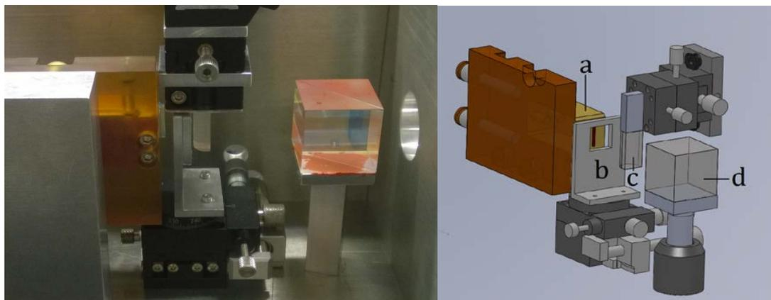
**Figure 6.** A picture the laser-box (left) of the current volume Bragg grating narrowed laser configuration, CAD drawing (right); a) laser diode, b) support for the optical grating, c) cylindrical lens, d) beam splitter.
