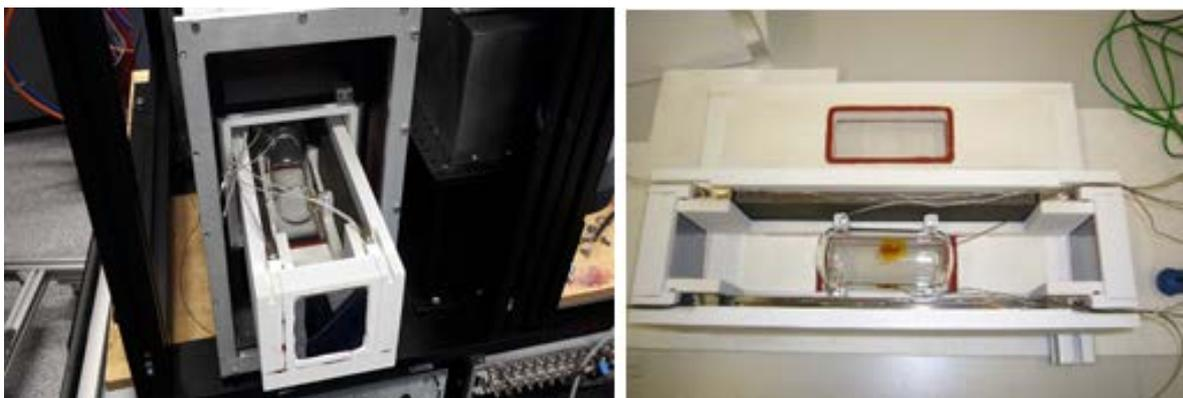
**Figure 4.** The new oven with  $^3\text{He}$  cell inside the magnetic cavity
