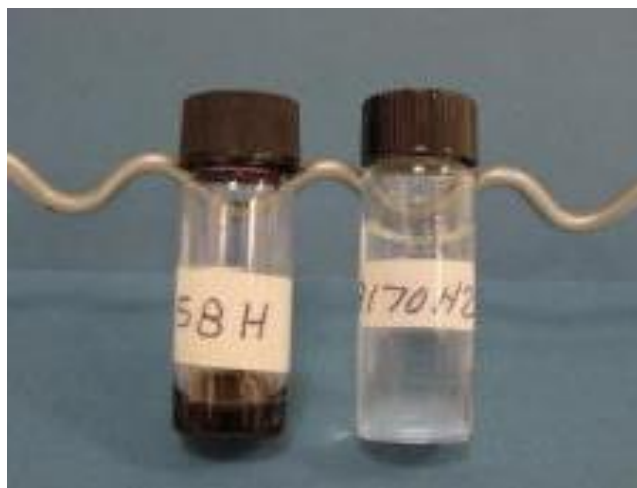
Figure 4. Photographs showing vials with different technical grades of sulfur mustard: On the right, a vial is shown with pure sulfur mustard as a clear, transparent liquid; On the left, a vial is shown containing sulfur mustard as a dark liquid due to impurities from production reaction. Reproduced with permission from Bundeswehr Institute of Pharmacology and Toxicology Munich, Germany 49 .
